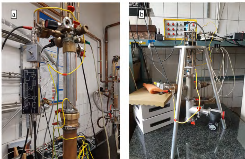
Figure 3.5: Sample holders during measurements. (a) Low-temperature measurement setup. The room-temperature part of the sample-holder has all the connection outlets. During measurements, proper grounding is important, otherwise the noise level would be high. (b) Room-temperature measurement setup during a measurement. This setup is more compact, but has the same connection outlets. The setup is placed on a vibration isolation platform.
