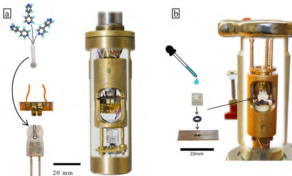
Figure 3.6: Photomontage of the measurement setup illustrating molecule dosage techniques. (a) In situ evaporation of molecules. The sample is placed into the sample holder, as seen on the right. A small quartz tube is filled with the target molecule and placed inside the tungsten filament of a small light bulb, which is then placed below the sample for evaporation. [40] (b) Molecule dosage in solution using a liquid cell. [40]
