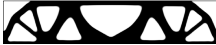
Figure 4.5: Optimal design in case of uncorrelated forces ( CV = 0.25 for all forces, P_{fail} = 0.1 ), V/V_0 = 0.497 .
