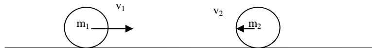
Figure 10.2 shows two particles of masses, m_1 and m_2 , and velocities, v_1 and v_2 , before they collide (1-D collision)
