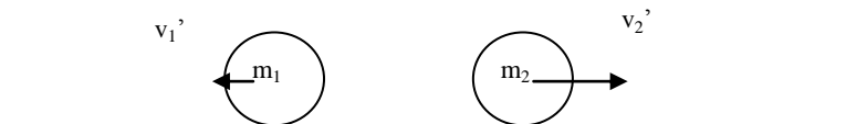
Figure 10.3 shows two particles of masses, m_1 and m_2 , and velocities, v_1' and v_2' , after they have collided (1-D collision)
