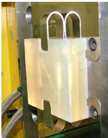
Fig 4 Assembled and fastened injection mold fastened on the stationary mold platen of an injection mold machine
