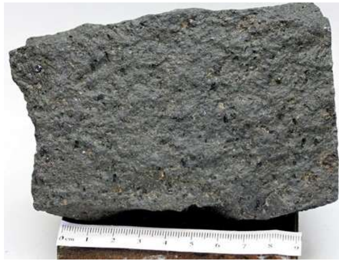
Figure 6: Porphyritic structure of extrusive igneous rocks (basalt).
