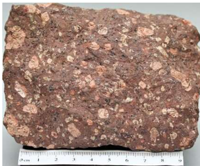
Figure 5: Porphyritic structure of intrusive igneous rocks (granite porphyry).
