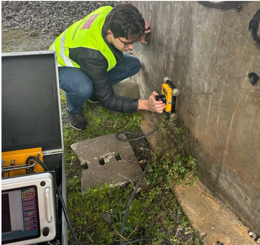
Figure 2. Visual inspection using Ground Penetrating Radar
