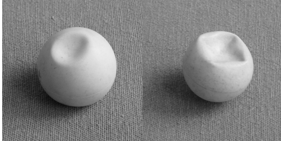
Figure 1.9.: Buckling shapes of a ping-pong ball: circular shape at smaller deflection, polygonal shape at larger deflection (photo by the author)
