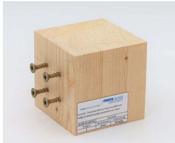
Fig. 5. Test specimen of reinforced timber
