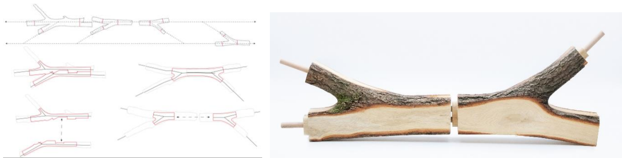
Fig. 7. Parts of a Raw-Timber-Truss with Off-Knot-Joints
