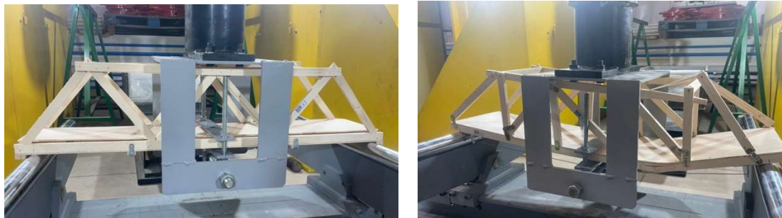
Figure 3: Loading test at the semifinal.
