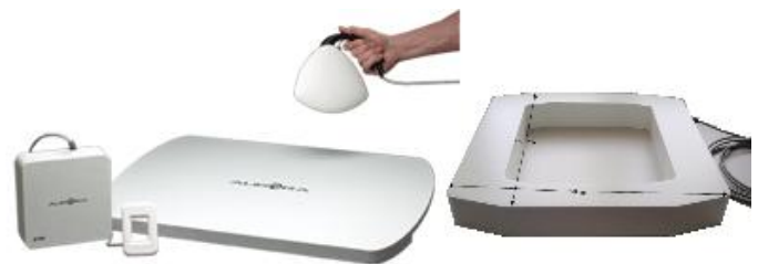
Fig.2. The different types of EMT field generators (Developed for the NDI Aurora system.)
