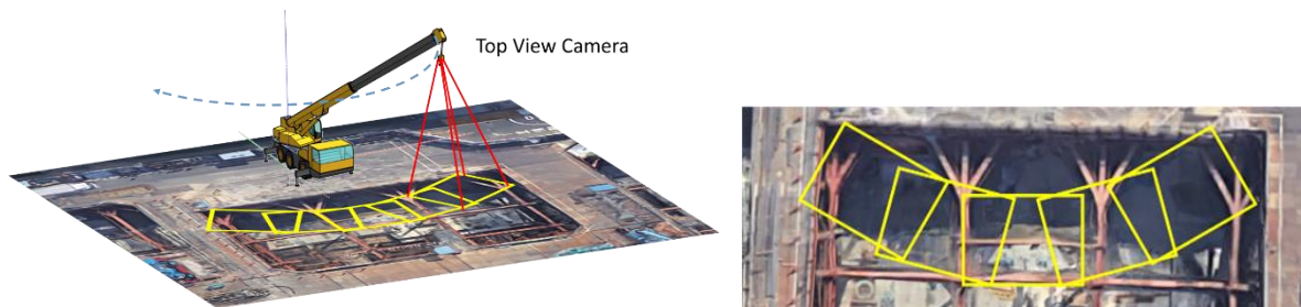
(a) Top-view camera surveying workspace
