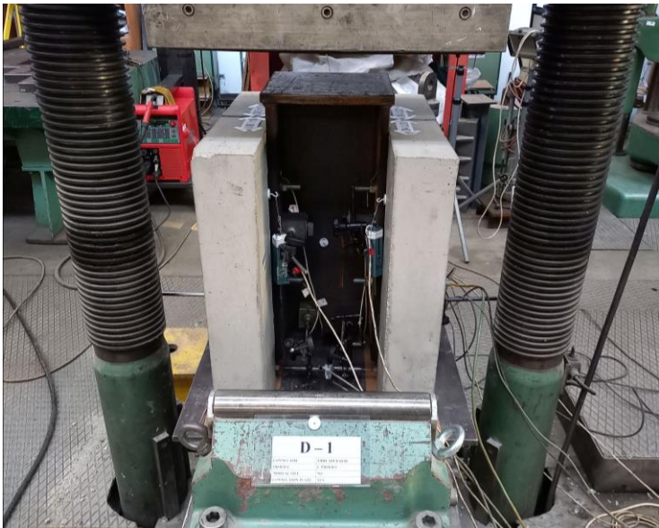
Figure 4. The prepared push-out test specimen
