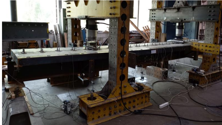
Figure 11. Test setup with specimen DC4-G – loading frames and measurement equipment
