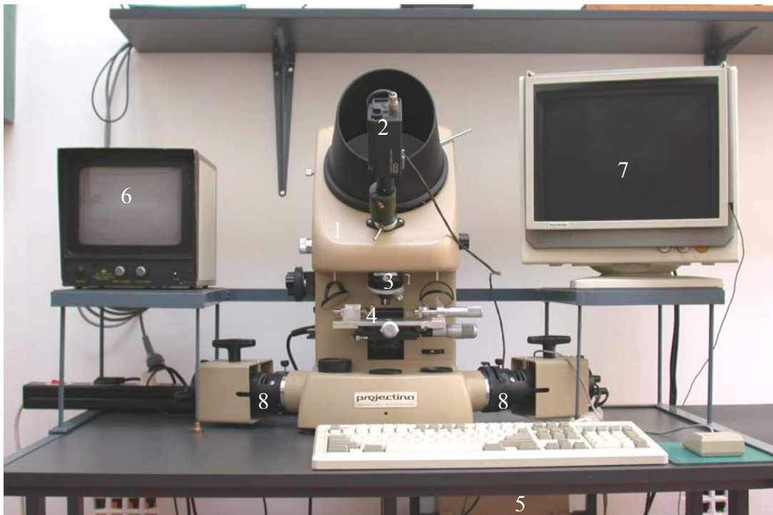
Figure 31 The image processing system at our Department (1-Projectina 4011-4016/MMA, 2-CCD video camera, 3- objective, 4- specimen, 5 Computer, 6- real-time monitor, 7- SVGA monitor, 8- quartz-iodine lamp)
