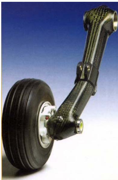
Figure 6 Braided composite helicopter landing gear by Eurocarbon [13]
