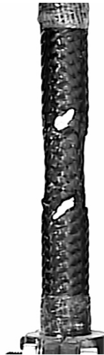
Figure 63 Neck-forming of tensile-loaded marked braided composite
