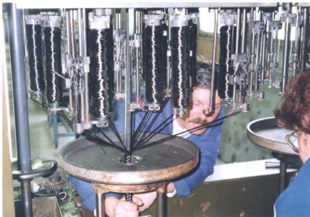
Figure 25 The beginning of braiding on a Steeger type braider (16 carriers)
