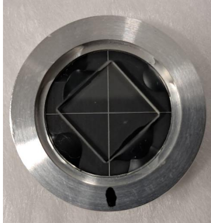
Figure 17. Aperture used for the alignment process of the photon pair source. The 50\ \mu\text{m} diameter pinhole is located at the center marked by the crosshair. The crosshair serves beam aiming purposes, while the glass plates in front of and behind the aperture provide an equivalent optical length for this device compared to that of the real BBO crystal.
