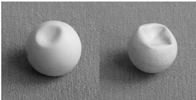
Figure 1.: Buckling shapes of a ping-pong ball: circular shape at smaller deflection, polygonal shape at larger deflection (photo by the author)
