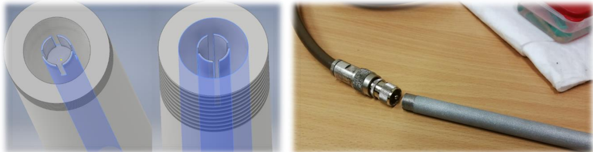
Fig. 115 Design and realization of 3D printed sensor for the determination of high frequency complex permittivity of dielectric liquids.
