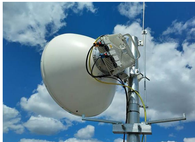
Figure 7. Antenna and E -band transceiver with Gbps optical ports.
