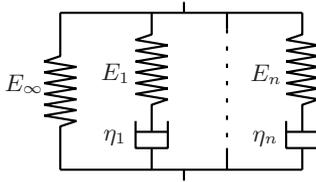
Figure 1: Generalized Maxwell model with parameters.
