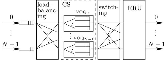
Figure 2: The overview of the load-balanced switch with  $N$  input and output ports
