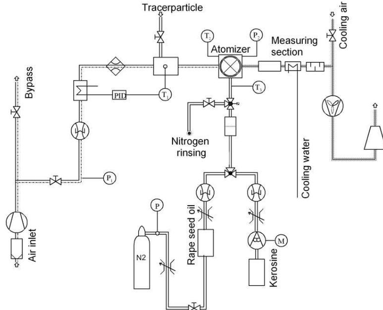
Fig. 1. Test rig to the research on the self-excited flames
