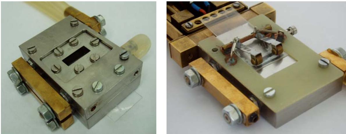
**Figure 1.** The sample holders of the rheoblock for SAXS and for freeze fracture
