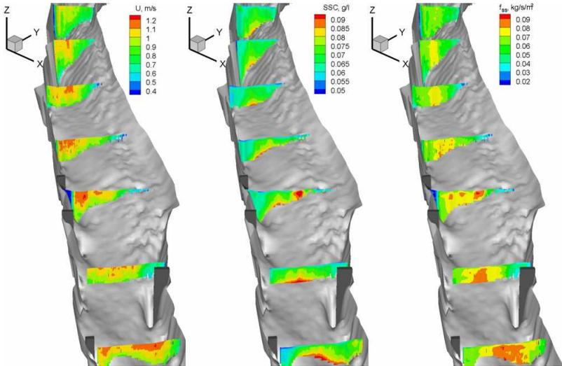
**Spatial distribution of measured flow velocities (left), derived sediment concentrations (mid) and calculated sediment fluxes (right).**
