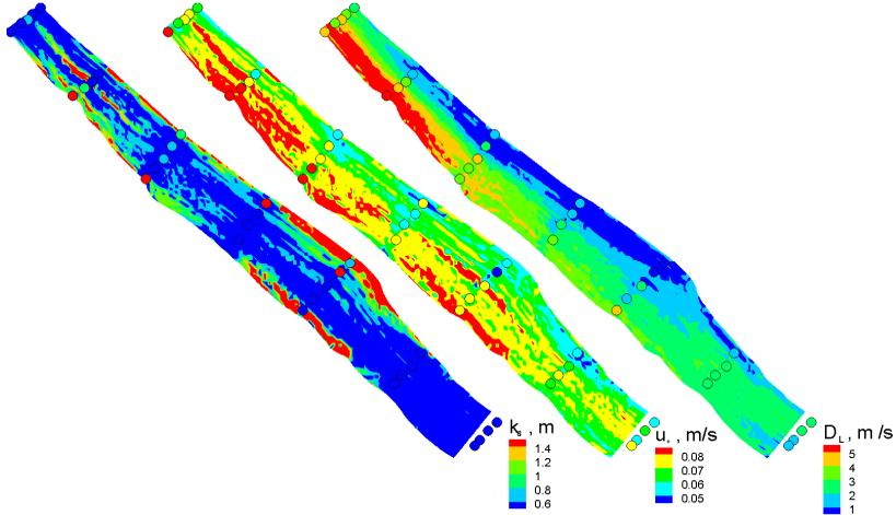
**Parameter distributions derived from ADCP data (left: Nikuradze roughness; mid: Bed shear velocity; right: Longitudinal dispersion coefficient).**
