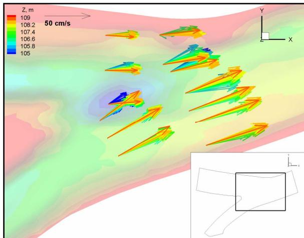
**Plan view of time averaged velocity vectors from fixed boat ADCP measurements.**
