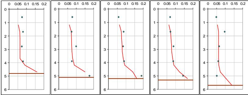
**Measured (dots) and estimated (lines) sediment concentration profiles
