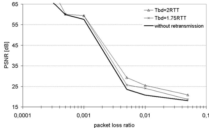
9. Figure Average PSNR of 150 seconds of 24 fps video as a function of packet loss
