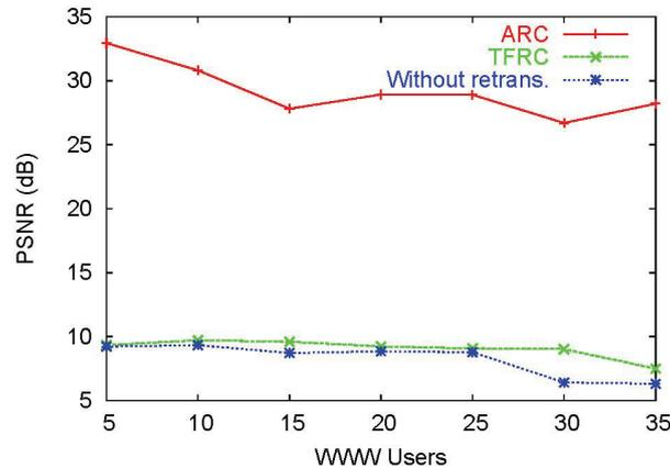
**5. Figure** Average PSNR without retransmission, with TFRC-based and ARC-based retransmission scheme (wireless loss is 10%)
