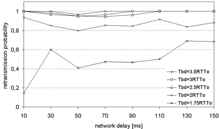
10. Figure The effect of playout buffer delay ( $T_{bd}$ ) on the retransmission probability
