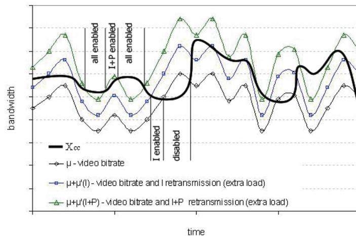
**6. Figure** The decision algorithm of the proposed CNRS retransmission method
