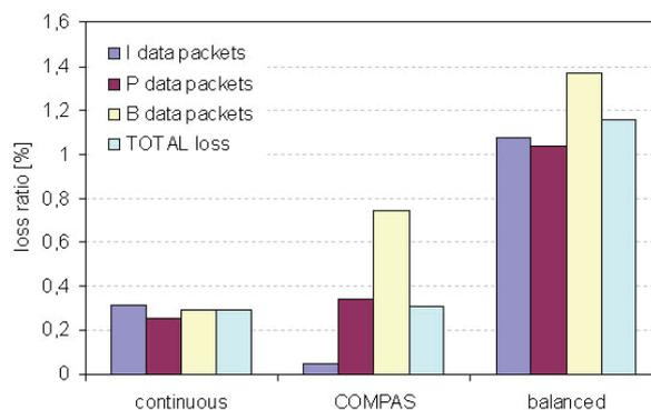
**12. Figure** Total and I-, P-, B-frame type data packet loss ratios
