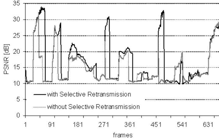
2. Figure Measured video quality in the DCCP/IP testbed
