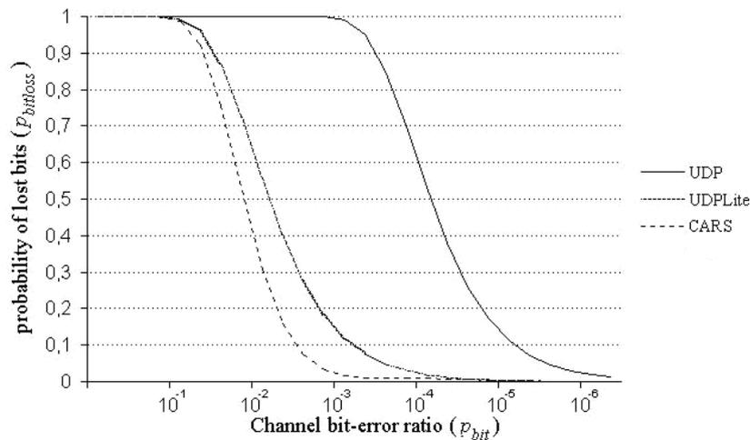
**1. Figure** Probability of damaged or lost bits in the MPEG stream in case of UDP, UDPLite and the proposed CARS algorithm
