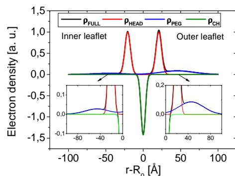
Fig. 4: The radial electron density profile of the studied sterically stabilized vesicles according to the model fits to the SAXS curves.
