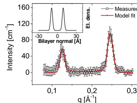
Fig. 1: The pure resonant curve of the DPPC/DBP system. The inset shows the distribution of the bromine atoms along the normal of the bilayer according to the model fitting.
