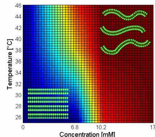
Fig. 3: The phase diagram constructed from the SAXS results of the DPPC/ $\text{CuCl}_2$  system. The colorbar represents the ratio of the well ordered (blue) and unbound (red) bilayers.
