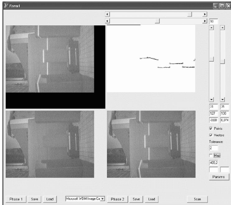
Figure 3.1. The user interface of the system. Input image with and without laser light on the bottom, blurred image on the top-left, the (rotated) result of the vectorization on the top-right
