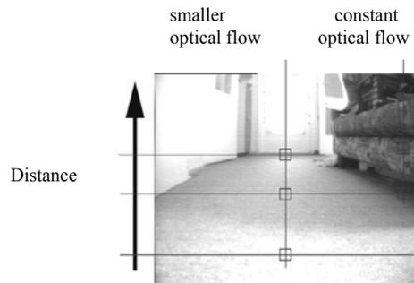
Figure 3.12. The principle of measuring depth data in a two-dimensional image
