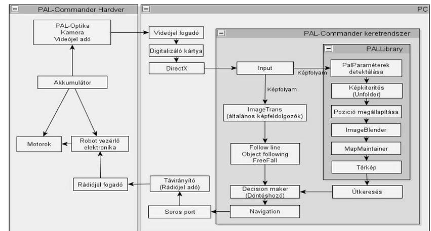
Figure 3.6. The PALCOM-system's modules and their relations
