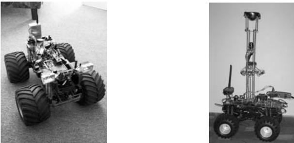
Figure 4.1. CCExplorer with forward looking traditional camera and with omnidirectional system
