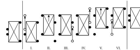
Figure 3.8. Movement strategy for one step forward, four-legged robot [VZ21]
