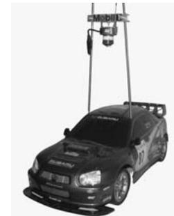
Figure 3.5. PALCOM mobile robot with PAL optics
