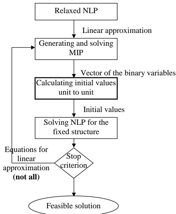
Figure 1. Modified Outer Approximation algorithm
