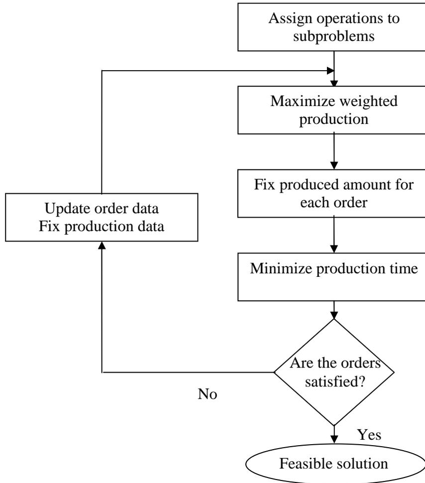
Figure 5. Scheme of the Rolling Operation algorithm
