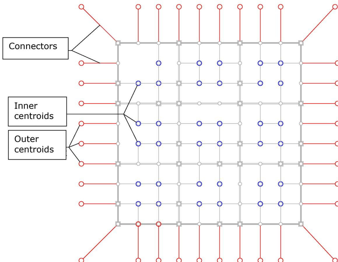
**Figure 1** Network model geometry
