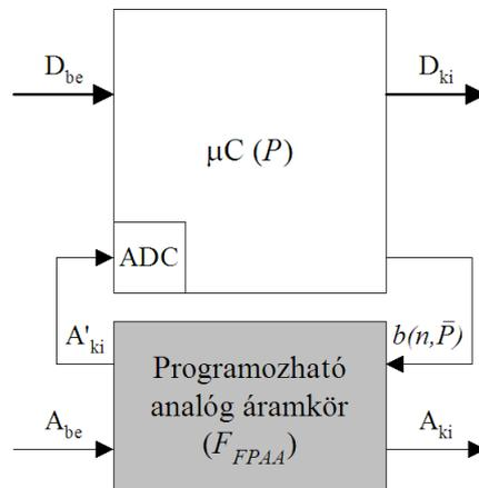
Figure 3: Feedback cooperation of the programmable analog circuit and the microcontroller.
