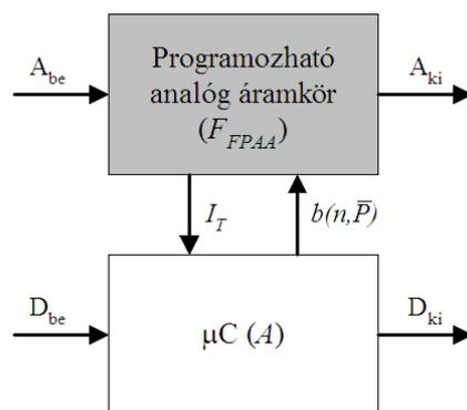
Figure 7: Connecting the microcontroller and the analog circuit with interrupt.
