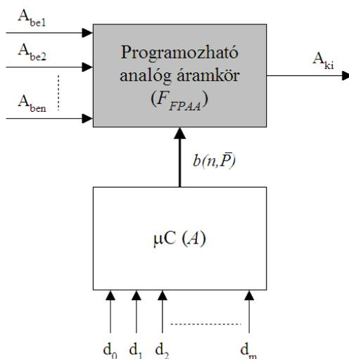
Figure 1: Controlling the circuit function of the programmable analog circuit with digital function.
