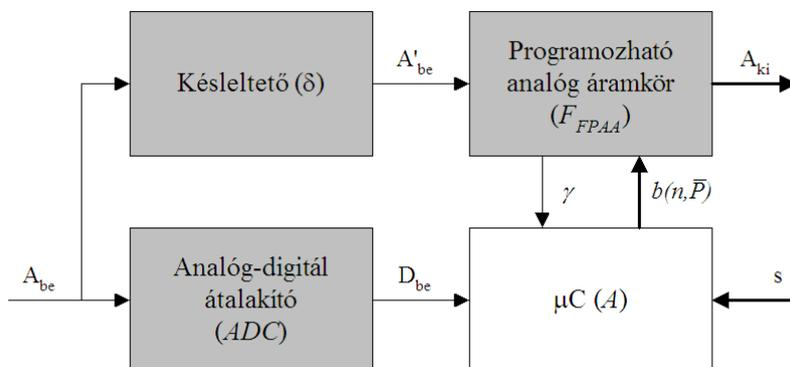
Figure 9: Constructing a robust electronic circuit with predictive control.
