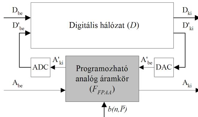
Figure 2: Feedback digital network through the outputs and inputs of the programmable analog circuit.
