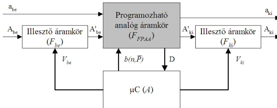
Figure 5: The programmable analog circuit with output and input attachment circuits in a microcontroller environment.
