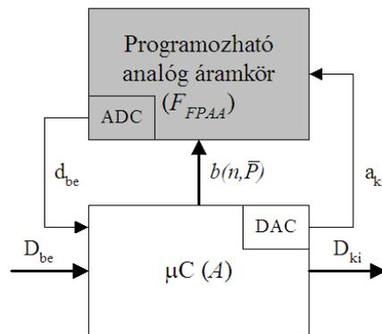
Figure 6: The programmable analog array as an analog signal processor cooperating with a microcontroller.
