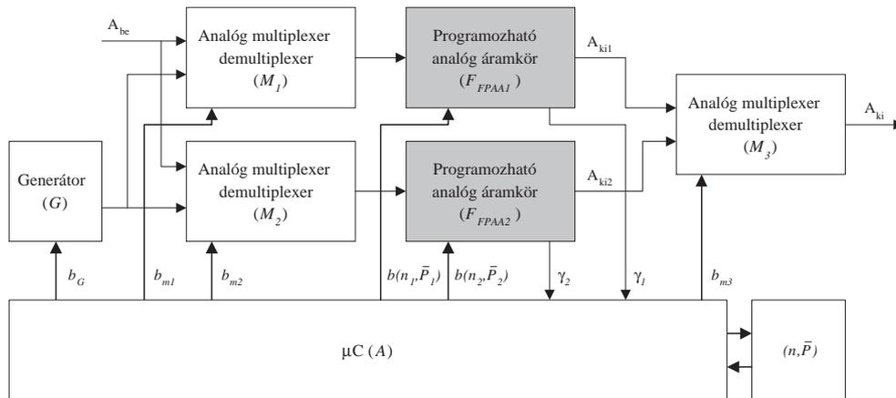
Figure 12: Measuring the transfer characteristics of the programmable analog circuit with a microcontroller in the background.
