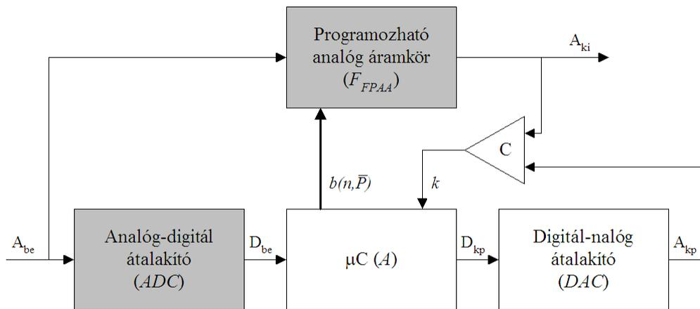
Figure 8: Making robust electronic circuits with a characteristic prediction.
