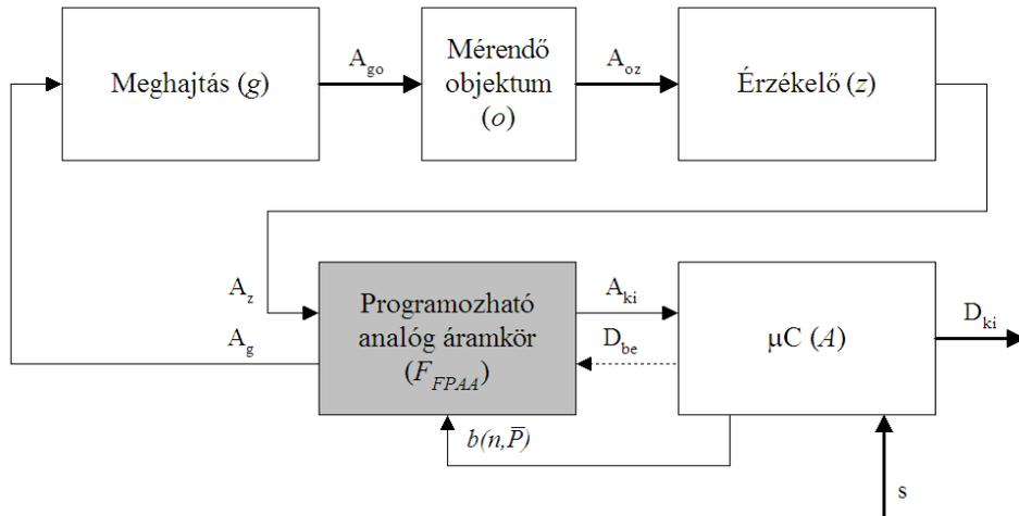
Figure 11: Constructing a self-adjust analog robust system in a measurement equipment.
