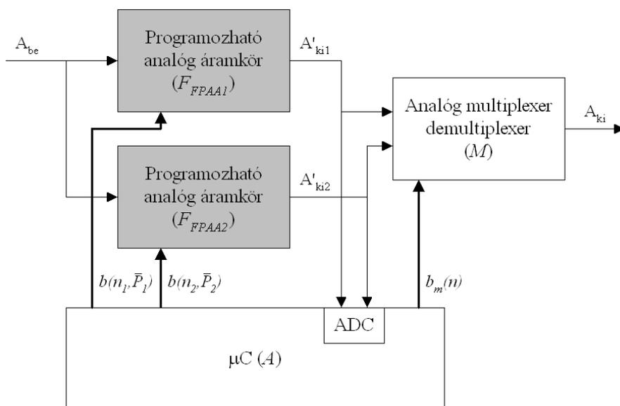
Figure 4: Circuit function change with microcontroller and programmable analog circuits.
