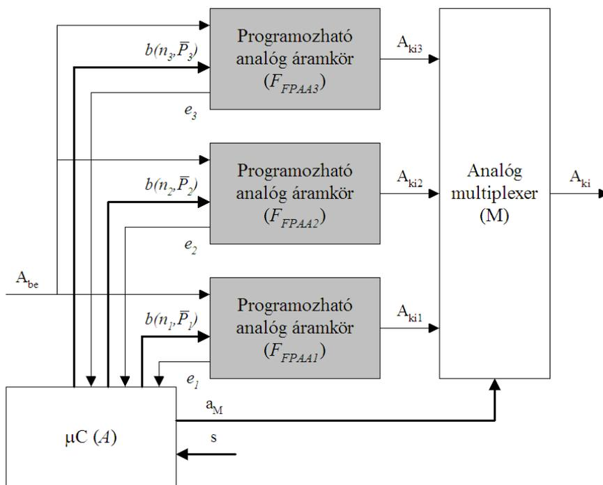
Figure 10: Majority voting principle error masking with programmable analog circuits and microcontroller.
