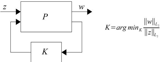
Figure 1: Control loop with plant  $P$  and controller  $K$ .  $K$  is designed to minimize the induced  $\mathcal{L}_2$  norm between  $w$  and  $z$ .
