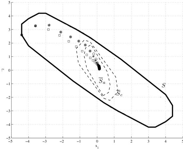
Figure 3: The maximal disturbance invariant sets (domains of applicability) of constant  $\mathcal{H}_\infty$  controllers ( $\bar{S}_a, \bar{S}_c$ ) and the disturbance invariant set of the interpolation based controller ( $S$ ) in a numerical example.
