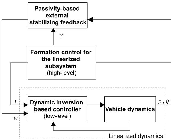
Figure 2: The simplified diagram of the dynamic inversion and passivity based control structure. ( $p, q$  are the position and velocity of the vehicles,  $V$  denotes the information required from the high-level controllers for the computation of the external feedback.)
