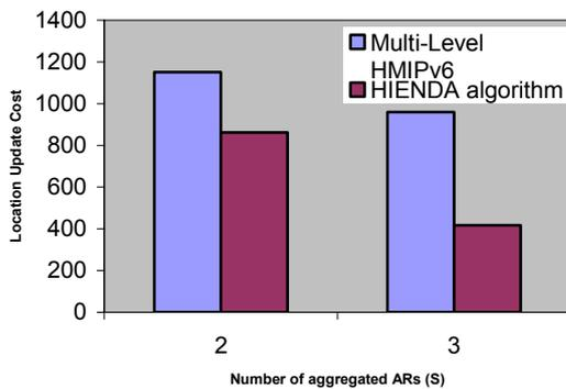
Figure 7 The Location Update Cost for the two hierarchical structures
