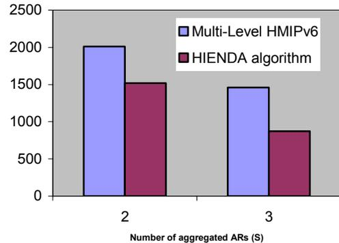
Figure 8 The Total Signalling Cost for the two hierarchical structures
