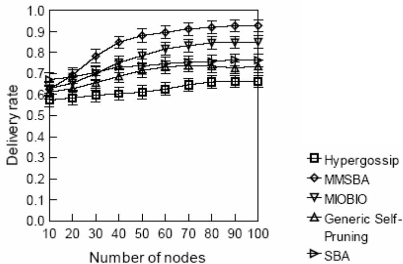
Figure 10 Delivery ratio of the simulated algorithms
