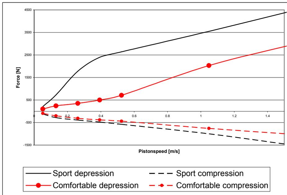
**1. ábra: Passive shock absorber characteristics**
