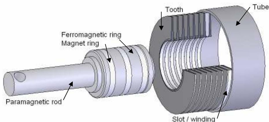
**2. ábra: Permanent magnetic synchronous tube machine (schematic draw)**
