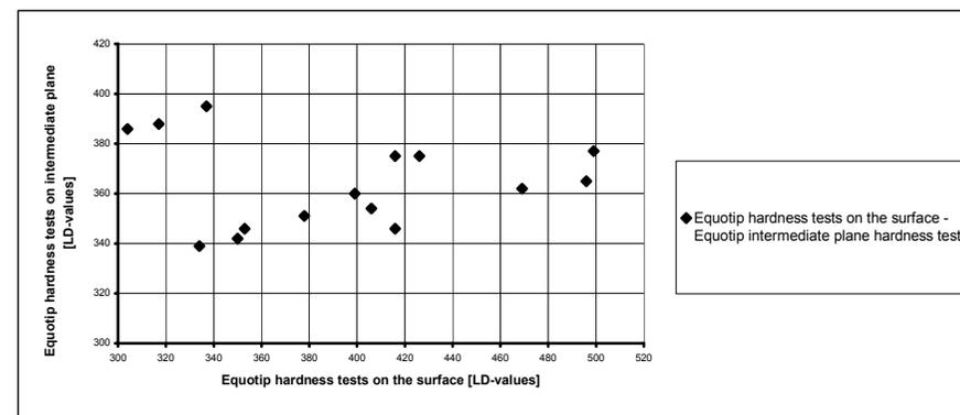
**Figure 5.** Searching for correlation between the strength values estimated from various harness tests
