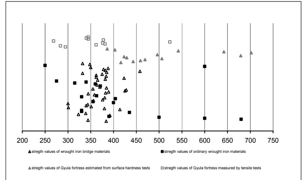
Figure 5. The strength values from the literature comparing with own test results
