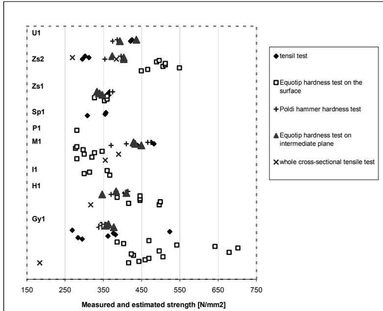
Figure 4. Strength data obtained by various methods
