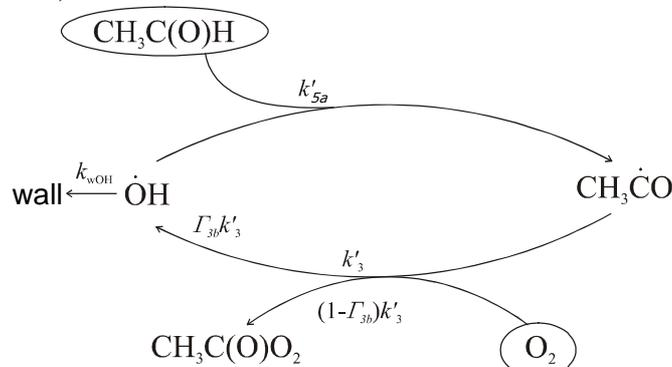
Figure 3. Reformation of  $\bullet\text{OH}$  in the  $\text{CH}_3\text{CO} + \text{O}_2$  reaction system.  $\Gamma_{3b} = k_{3b} / k_3$ ,  $k'_3 = k_3 \cdot [\text{O}_2]$ ,  $k'_{5a} = k_{5a} \cdot [\text{CH}_3\text{C}(\text{O})\text{H}]$ .
