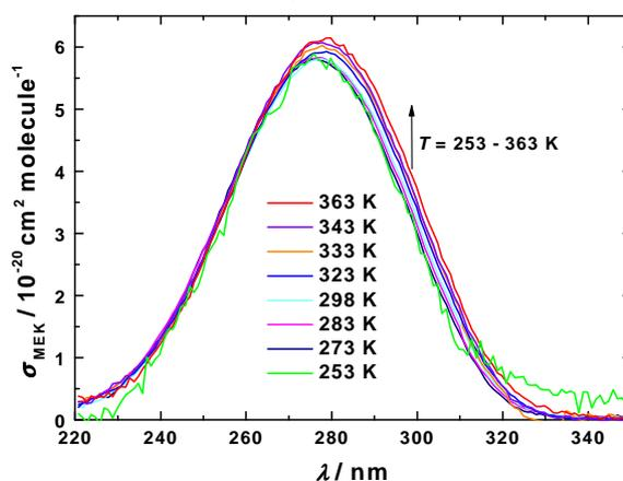
Figure 2. The UV-absorption spectrum of methyl-ethyl-ketone at different temperatures.
