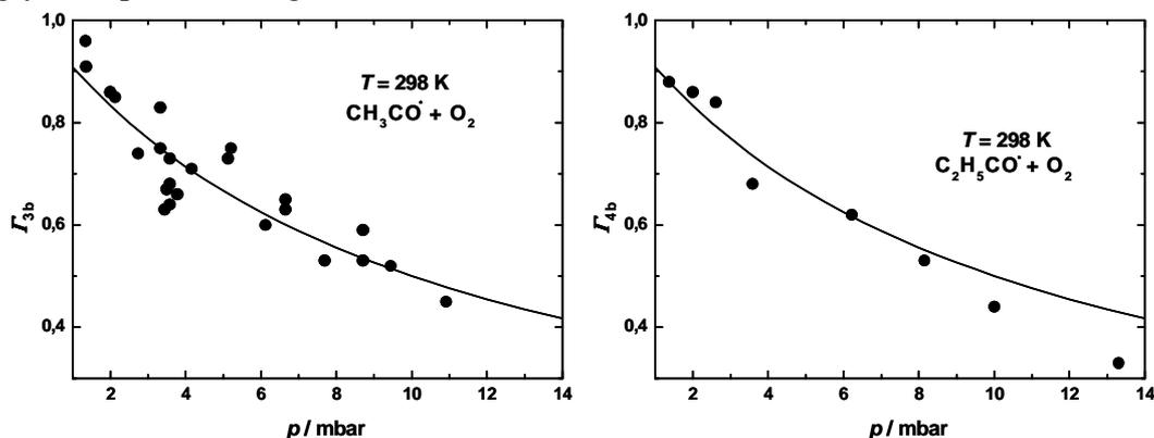
Figure 5. Pressure dependence of the  $\cdot\text{OH}$  product yield for the reactions of acetyl and propionyl radicals with  $\text{O}_2$  at room temperature in He buffer gas.
