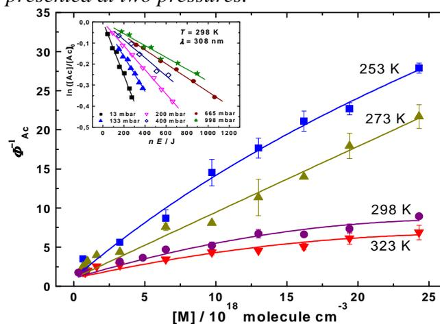
Figure 1. Stern-Volmer (SV) plots for the photodecomposition QY of acetone at  $\lambda = 308$  nm photolysis wavelength in synthetic air. The semilogarithmic decay plots in the insert show typical results of the evaluation of the experimental data according to eq. (1) to obtain  $\Phi_{Ac}$ .
