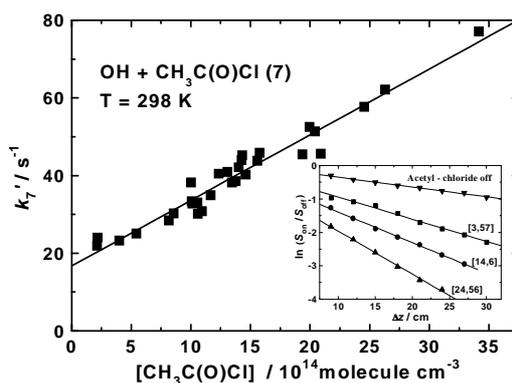
Figure 7. Plot of the pseudo-first-order rate constant vs. the acetyl-chloride concentration. The insert shows results according to eq. (6); in brackets  $\text{CH}_3\text{C}(\text{O})\text{Cl}$  concentrations are given in  $10^{14} \text{ molecule} \cdot \text{cm}^{-3}$ .
