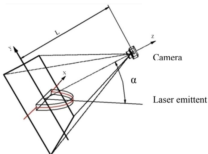
**Fig.1** Measurement principle
