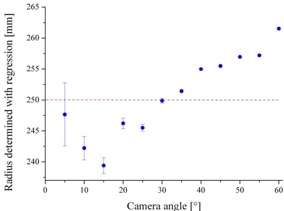
**Fig. 6** Radius determined with regression and deviation as a function of camera angle ( $\alpha$ )
