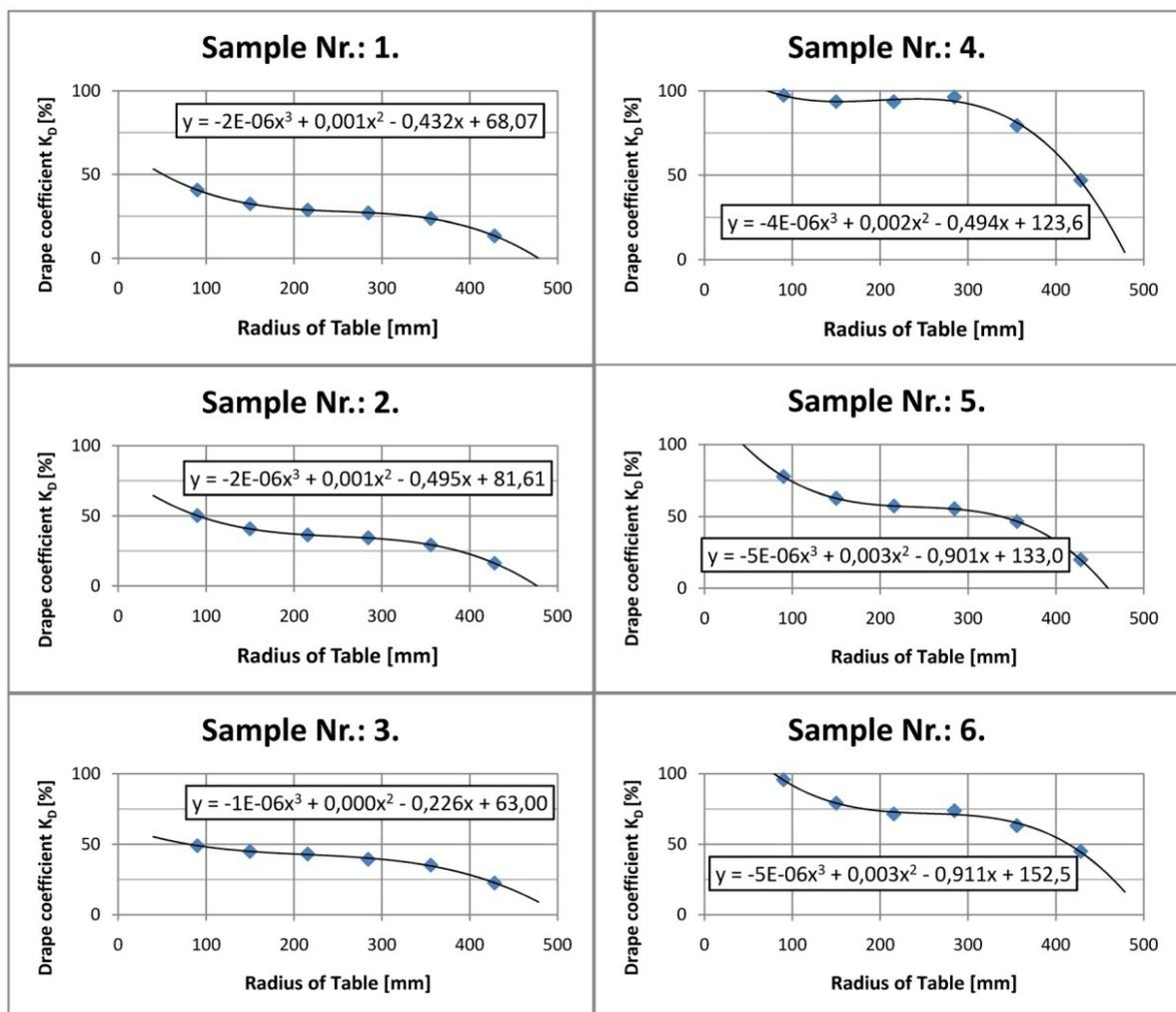
**Fig. 9** Drape coefficients as a function of table radius for different fabrics
