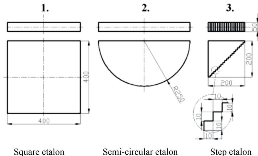
**Fig.2** Square and step-shaped calibration prism (1., 3.), and semi-circular control prism (2.)
