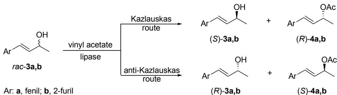
**Fig. 3:** Lipase catalysed kinetic resolution of the racemic (3*E*)-4-phenylbut-3-en-2-ol (*rac-3a*) and (3*E*)-4-(furan-2-yl)but-3-en-2-ol (*rac-3b*)
