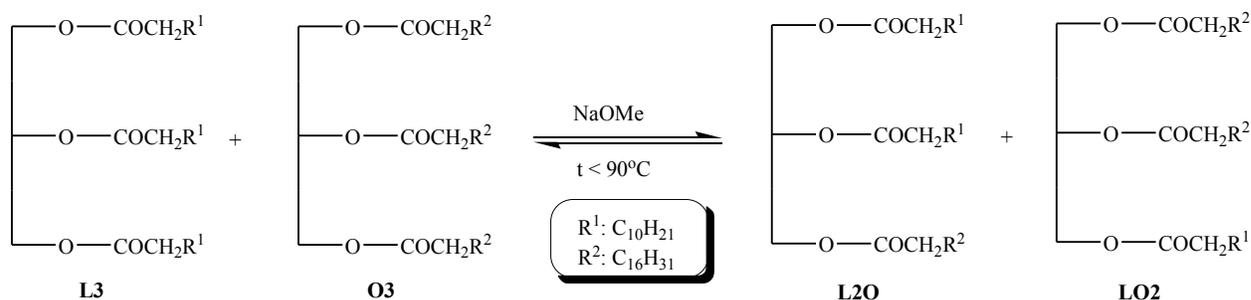
**Fig. 1:** Low temperature base catalysed interesterification reaction of triglycerols
