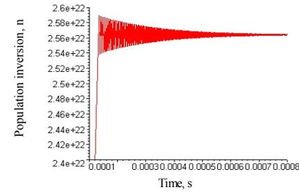
Fig. 1.5. Numeric result for the turn on transient of the population inversion density (pumping rate:  $W=0,7$ ).
