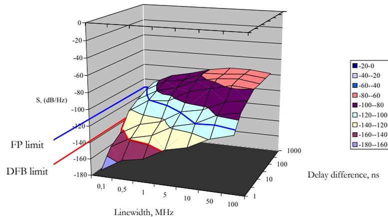
Fig. 2.6. Phase noise induced intensity noise at the UMZI output in case of different laser linewidth and interferometer delay difference value. The presented output power levels are valid at 0Hz off the optical carrier. Additionally I have marked the typical RIN levels for FP and DFB lasers ( $RIN_{FP} \approx -110 \text{ dB/Hz}$ ,  $RIN_{DFB} \approx -140 \text{ dB/Hz}$ ). In case of typical RIN levels noise suppression is possible at parameter combinations lying left from the limit line.
