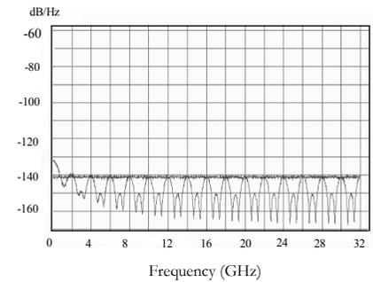
Fig. 3.3. Intensity noise reduction by a three tap filter. Above 3GHz the phase induced intensity noise is already smaller than the -140dB/Hz original laser noise level and thus at these frequencies periodic noise suppression is feasible. (laser linewidth: 2MHz)
