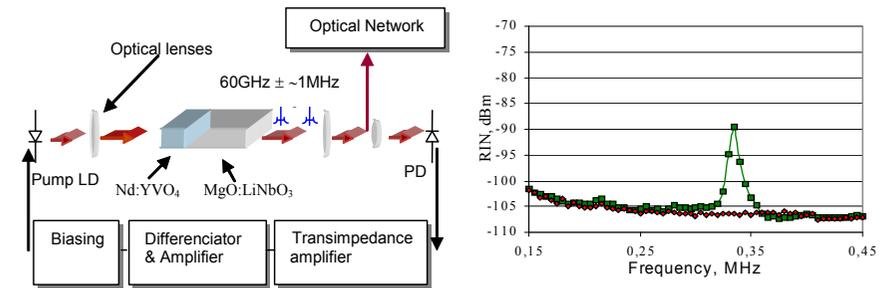
Fig. 1.3. Optoelectronic feedback loop in an optical transmitter containing Nd:YVO<sub>4</sub>
