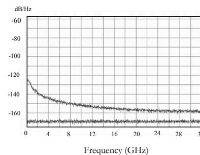
Fig. 3.4. Noise conversion having the laser carrier at the transfer function maximum.
