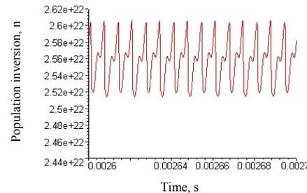
Fig. 1.9. Time variant solution for the population inversion density at a feedback modulation depth of 35%. The corresponding result for the photon density is a similar period doubling bifurcation.
