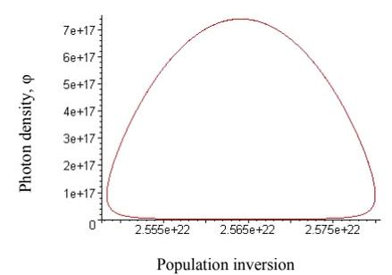
Fig. 1.8. Solution of the time variant nonautonomous rate equations at a modulation depth of 25%. The phase portrait depicts a limit cycle.
