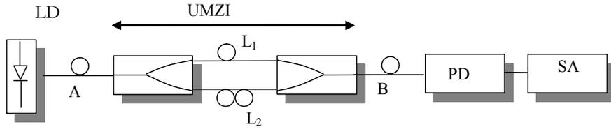
Fig. 2.1. Unbalanced Mach-Zehnder Interferometer (UMZI) depicted between A and B. In this measurement setup the output signal of the laser diode (LD) is passing through the UMZI. The output is detected by a photodiode (PD) and further processed by a spectrum analyzer (SA).
