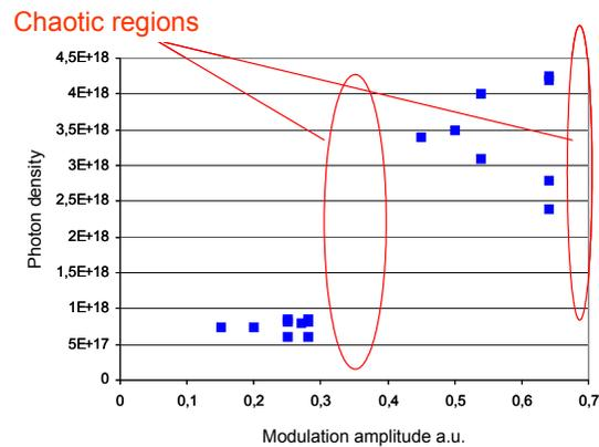
Fig. 1.13. Bifurcation diagram of a Nd:YVO<sub>4</sub> laser.
