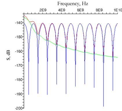
Fig. 2.2. Output spectral density in case of 20MHz linewidth DFB (Distributed Feedback Laser) laser (RIN=-140dB/Hz) and 1ns delay difference UMZI. Blue curve: intensity noise induced output intensity, green curve: phase noise induced intensity noise, red curve: resultant noise level.
