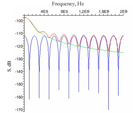
Fig. 2.3. Output spectral density in case of 20MHz linewidth Fabry-Perot laser diode (RIN=-110dB/Hz) and 5ns delay difference UMZI. Blue curve: intensity noise induced output intensity, green curve: phase noise induced intensity noise, red curve: resultant noise level.
