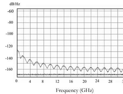
Fig. 3.2. Phase noise induced intensity noise at the output of 2MHz linewidth laser driven three tap optical filter (delay difference: 0.5ns, RIN=-170dB/Hz)
