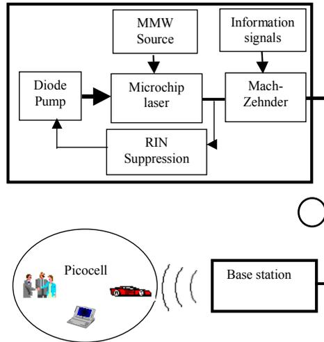
Fig. 1.1. Solid-state laser based optical-mobile system
