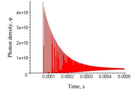
Fig. 1.6. Numeric result for the turn on transient of the photon density (pumping rate:  $W=0,7$ ).
