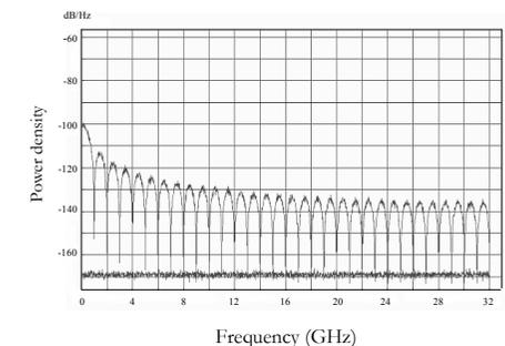
Fig. 3.5. Noise conversion having the laser carrier at the transfer function's -3dB point.
