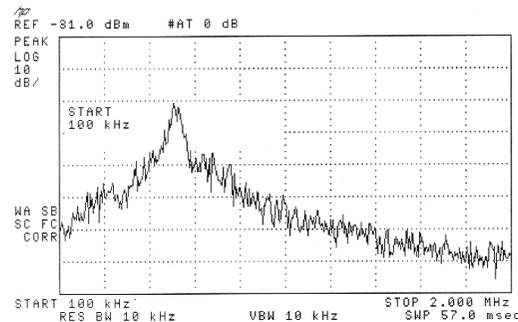
Fig. 1.2. Nd:YVO<sub>4</sub> laser intensity noise peak (relaxation oscillation frequency: 500kHz, optical pump power: 100mW).
