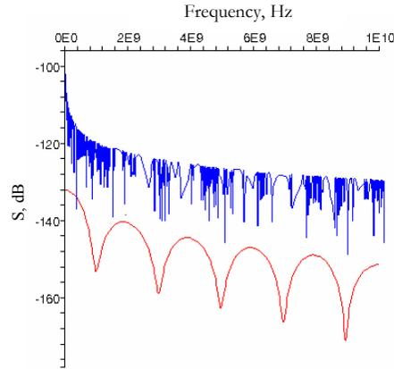
Fig. 3.1. The calculated output power density at the output of a three tap transversal optical filter induced by the input laser phase noise. (the filter coefficients present a uniform distribution, attenuation was neglected). The upper (blue) curve is for the incoherent case ( $\tau=0.5\mu\text{s}$ ), the lower (red) curve stands for a coherent setup ( $\tau=0.5\text{ns}$ ).
