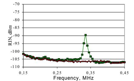
Fig. 1.4. The observed noise suppression at the relaxation oscillation frequency of the Nd:YVO<sub>4</sub> solid-state laser.
