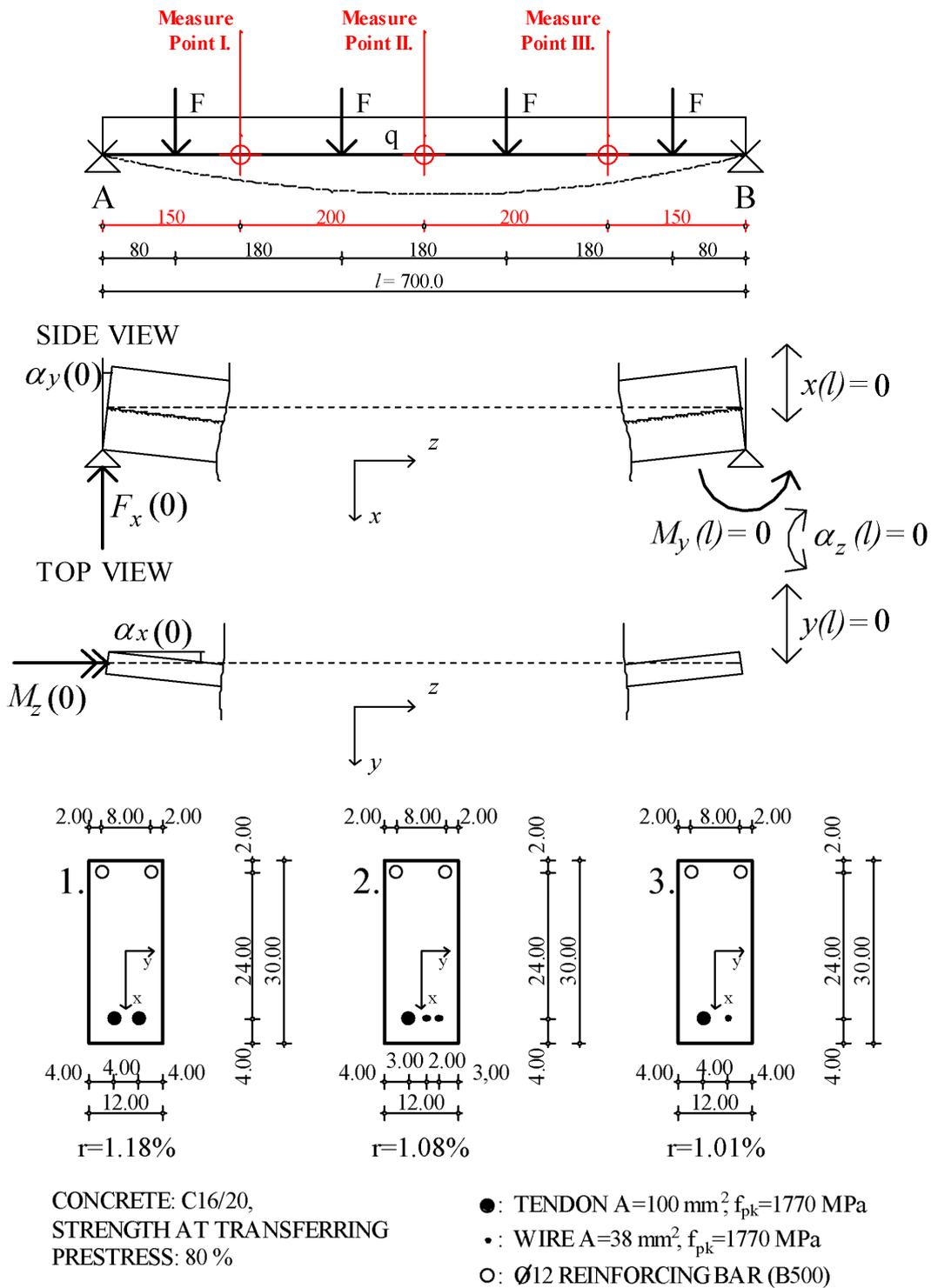
Figure 2: The simply supported beam of the experiments, measures are in cm
