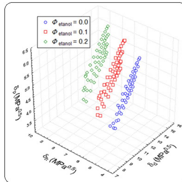
Figure 9. The Hansen-diagram for the  $\text{CO}_2$ -ethanol mixtures for the technologically relevant domain.
