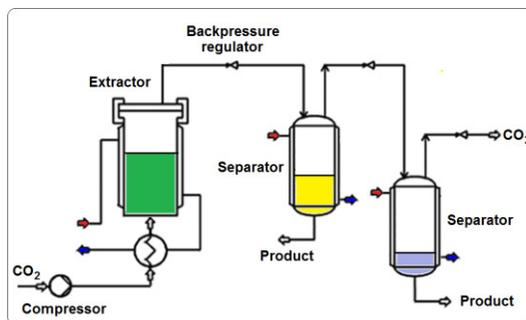
Figure 1. Scheme of supercritical fluid extraction pilot plant.
