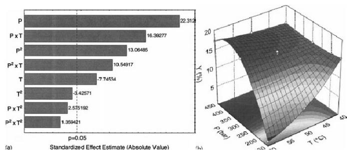
Figure 3. The influence of extraction parameters (pressure ( $P$ ) and temperature ( $T$ )) on oil yield ( $Y$ ):(a) Pareto diagram, (b) the response surface of oil yield
