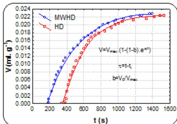
Figure 7. The comparison of the essential oil obtaining kinetics for HD and MWHD
