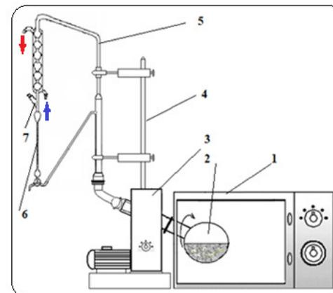
Figure 2. The scheme of the microwave-assisted hydro-distillation apparatus: 1- microwave oven, 2- spherical flask, 3- rotating evaporator, 4- supporting rack, 5- Clevenger-head, 6- scaled tube, 7- safety valve / snap stopper.
