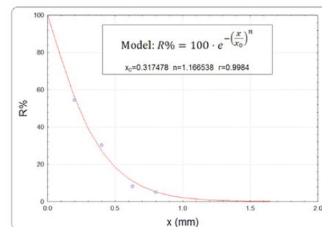
Figure 4. The fitted values of the particle size distribution parameters.
