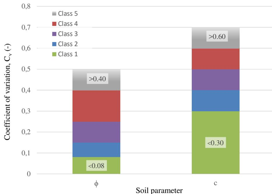
Figure. 1. Quality classes offered for internal friction angle and cohesion
