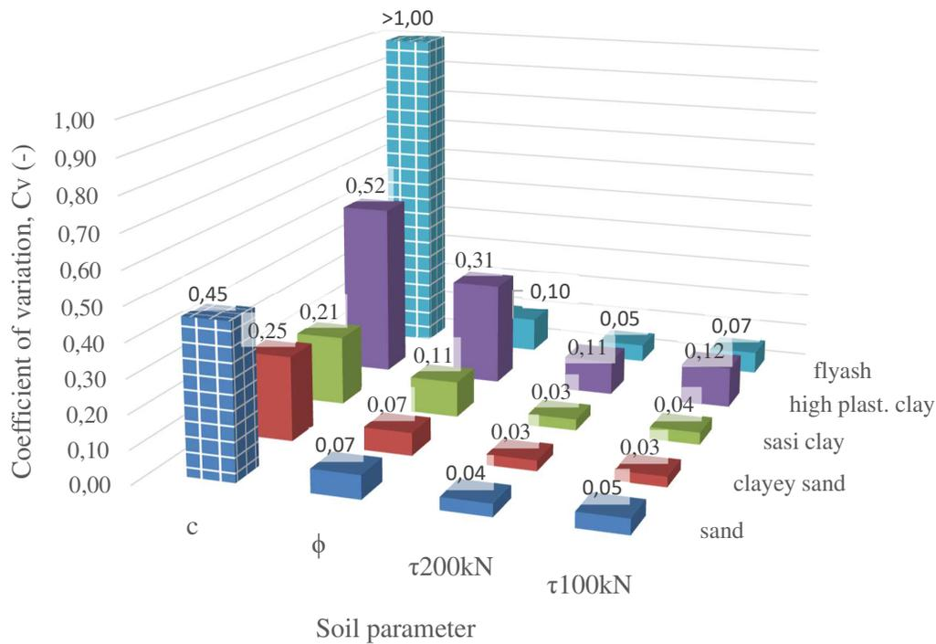
Figure 3. Coefficient of variation values of shear strength and shear strength parameters in case of different soils
