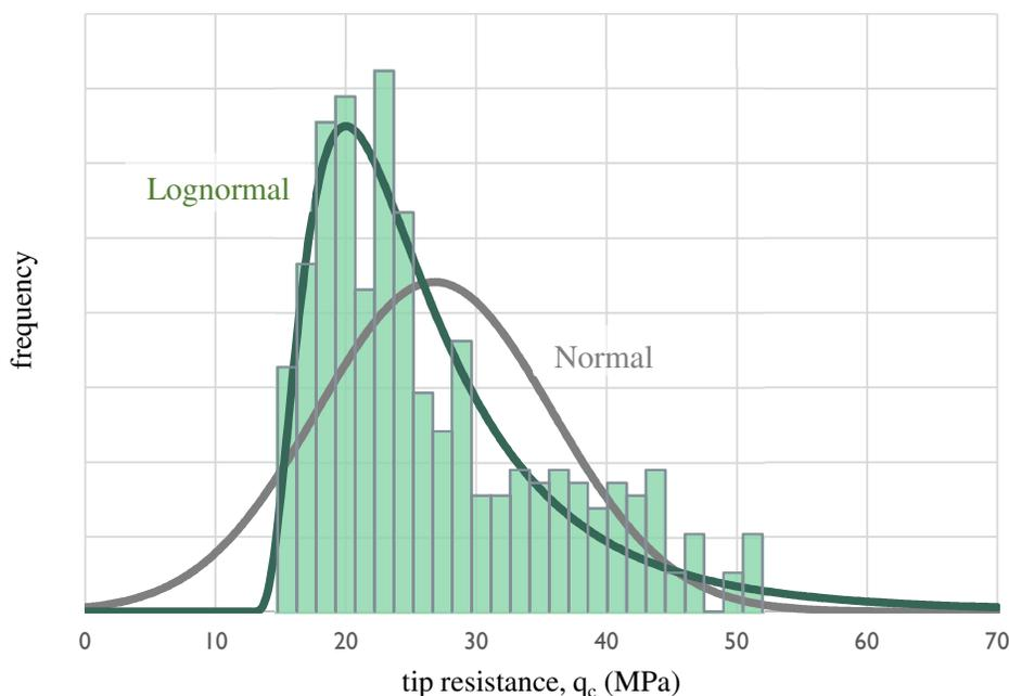
Figure 4. Example for fitting Normal and Lognormal distribution function on CPT tip resistance measurements
