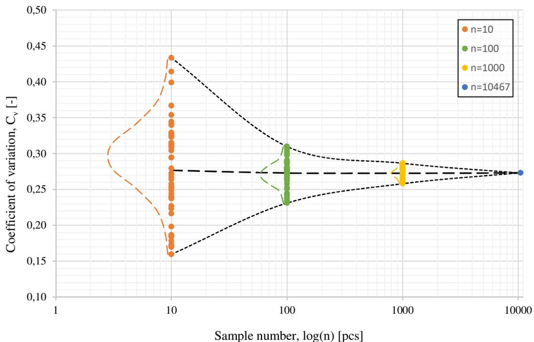
Figure. 2. Coefficient of variation values determined based on different sample numbers in case of Pleistocene medium sand layer
