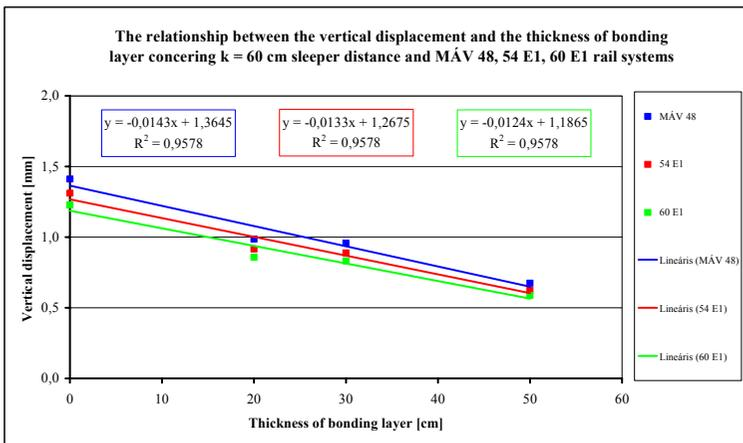
**Figure 5:** The determined tight relationship between the vertical displacement and the thickness of bonding layer concerning  $k = 60$  cm sleeper distance and MÁV 48, 54 E1, 60 E1 rail systems
