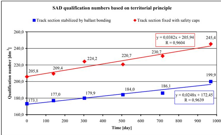
Figure 11: The determined SAD qualification numbers in the track section stabilized by ballast bonding and in the track section fixed with safety caps
