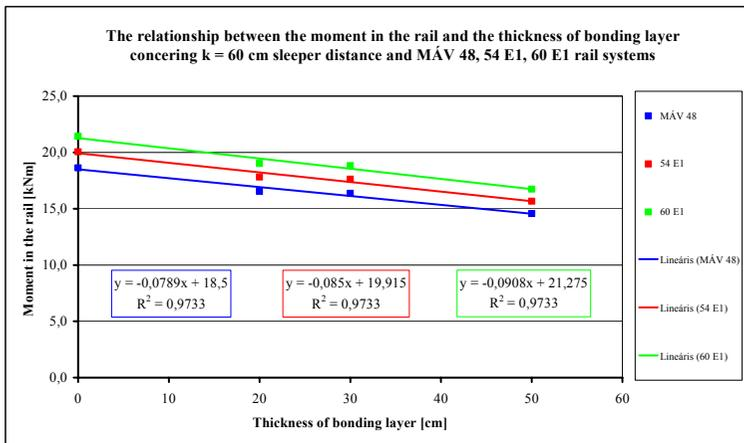
Figure 7: The determined tight relationship between the moment in the rail and the thickness of bonding layer concerning  $k = 60$  cm sleeper distance and MÁV 48, 54 E1, 60 E1 rail systems
