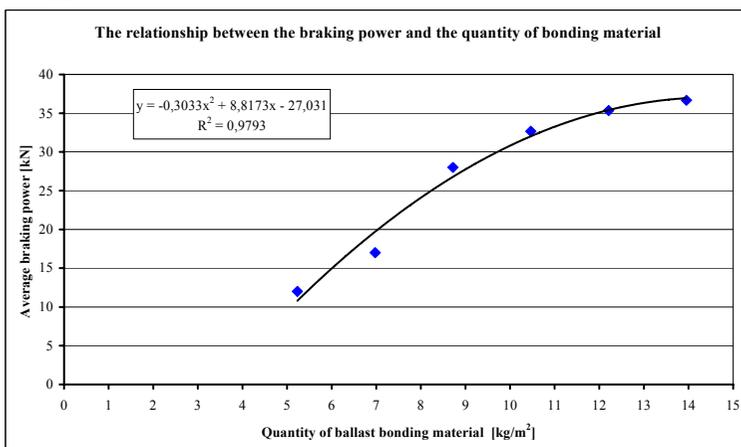
Figure 1: Tight relationship between the braking power and the quantity of bonding material.
