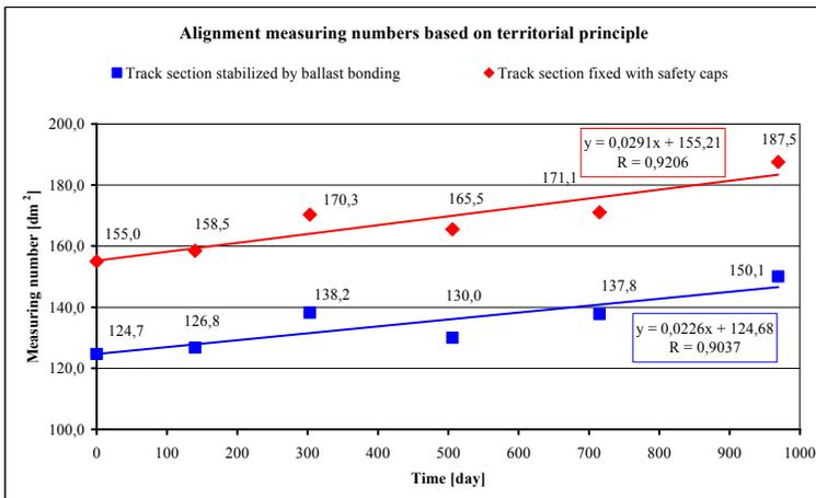
Figure 12: The determined alignment measuring numbers in the track section stabilized by ballast bonding and in the track section fixed with safety caps
