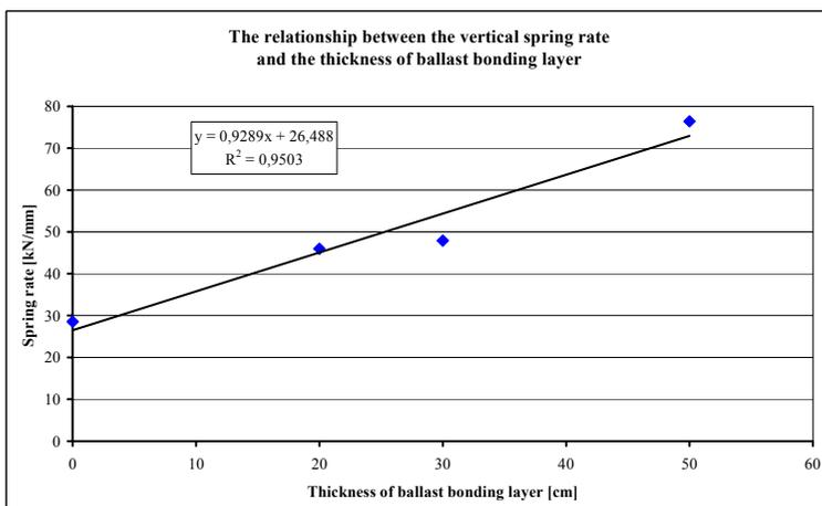
**Figure 3:** The determined tight relationship between the vertical spring rate and the thickness of ballast bonding layer
