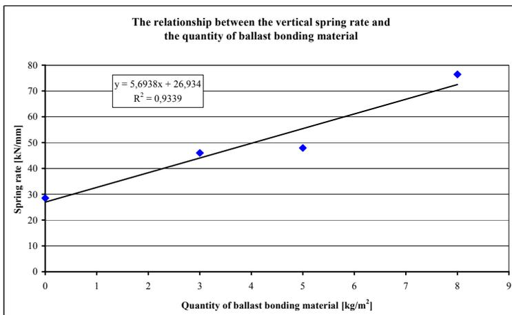
**Figure 2:** The determined tight relationship between the vertical spring rate and the quantity of ballast bonding material
