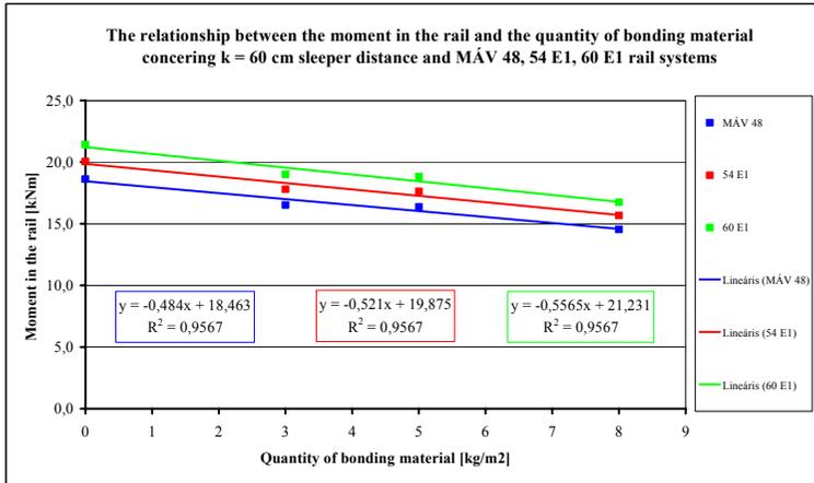
Figure 6: The determined tight relationship between the moment in the rail and the quantity of bonding material concerning  $k = 60$  cm sleeper distance and MÁV 48, 54 E1, 60 E1 rail systems
