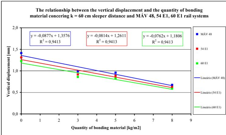
**Figure 4:** The determined tight relationship between the vertical displacement and the quantity of bonding material concerning  $k = 60$  cm sleeper distance and MÁV 48, 54 E1, 60 E1 rail systems
