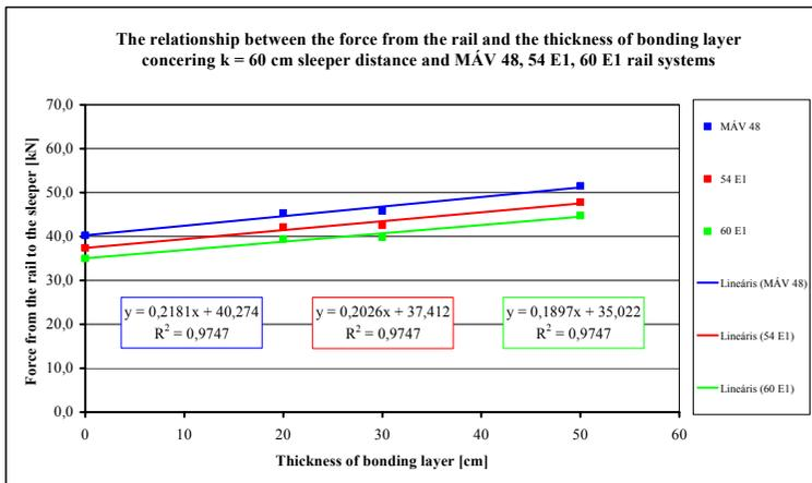
**Figure 9:** The determined tight relationship between the force from the rail and the thickness of bonding layer concerning k = 60 cm sleeper distance and MÁV 48, 54 E1, 60 E1 rail systems
