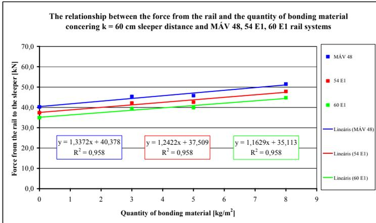
**Figure 8:** The determined tight relationship between the force from the rail and the quantity of bonding material concerning k = 60 cm sleeper distance and MÁV 48, 54 E1, 60 E1 rail systems
