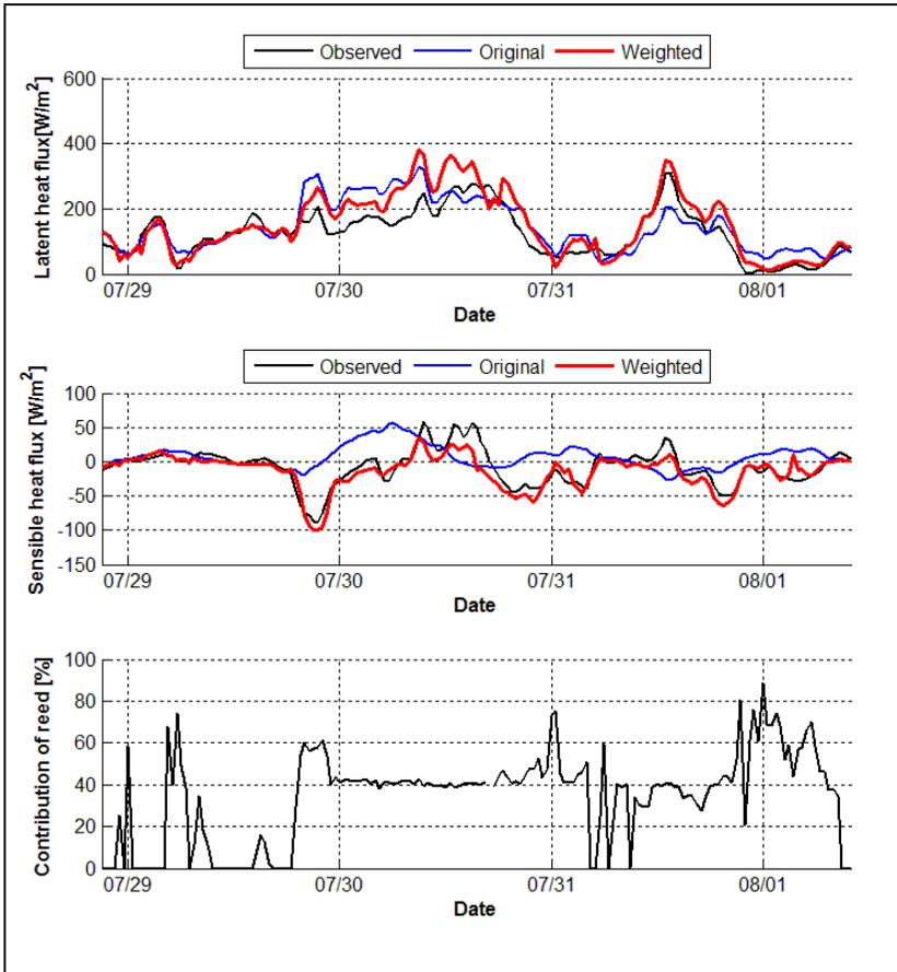
**Observed, modeled (original) and weighted sensible and latent heat flux at the open water zone along with the footprint contribution of the reed zone in a representative period**
