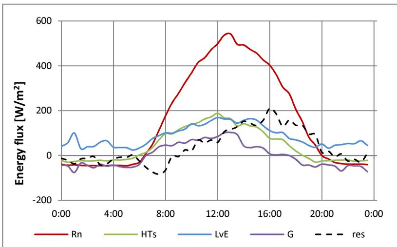
**Mean diurnal course of the energy budget terms of the reed zone averaged in May 2013. Notation:  $R_N$  – net radiation,  $HT_S$  – sensible heat flux,  $L_{vE}$ – latent heat flux,  $G$  – storage term and  $res$  – residual**
