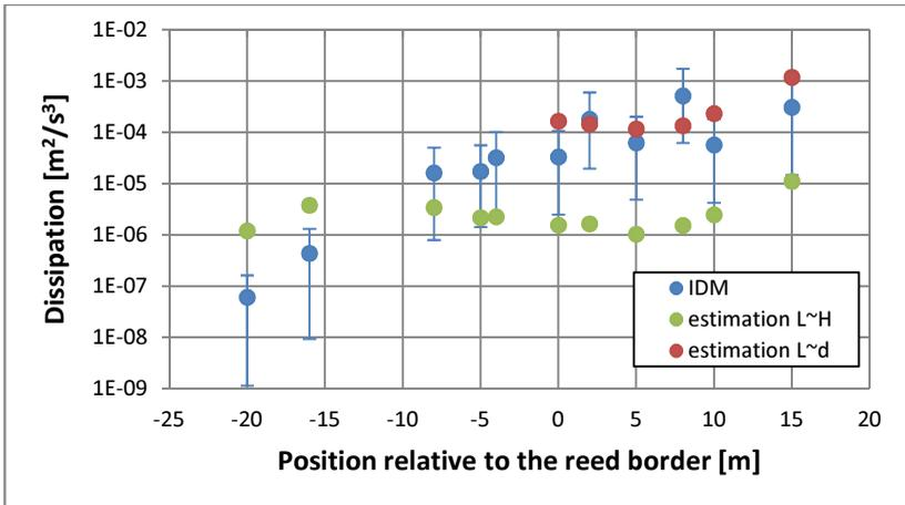
**Energy dissipation rate derived from the inertial dissipation method (IDM) and the theoretical formula according to Tennekes and Lumley (1972) versus the position relative to the reed border. Notation:  $L$  – characteristic length scale,  $H$  – water depth,  $d$  – average stem diameter**
