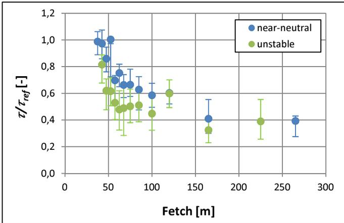
**Normalized wind shear stress above open water along the fetch. The base of normalization is the reference wind speed measured by the fixed anemometer of the reed station**
