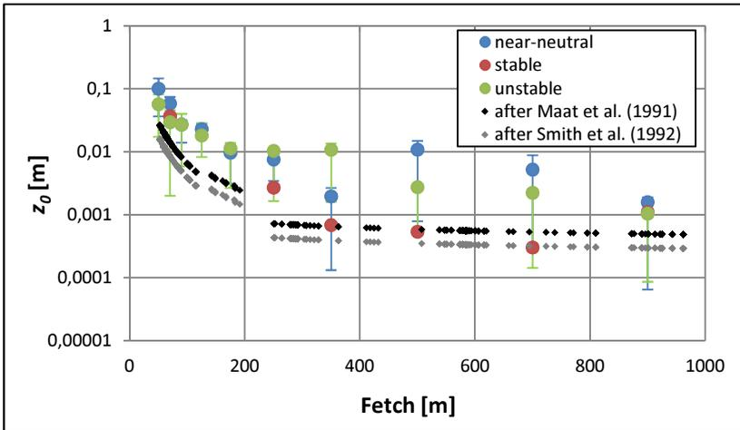
**Roughness length of open water as a function of fetch estimated from the logarithmic profile formula (dots colored after stability conditions) and from wave age relations (black and grey rhombuses)**
