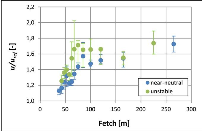
**Normalized horizontal wind speed above open water along the fetch. The base of normalization is the reference wind speed measured by the fixed anemometer of the reed station**
