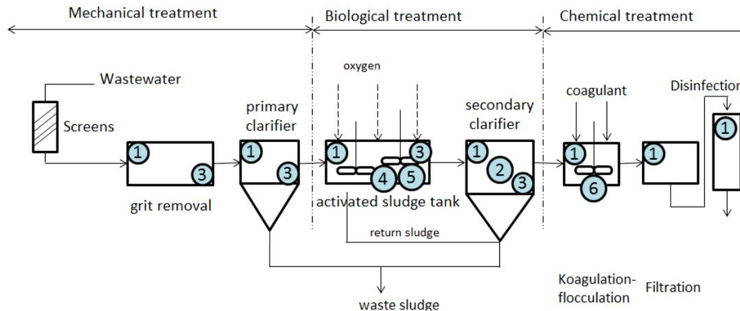
Figure 1: The overall scheme of the wastewater treatment
