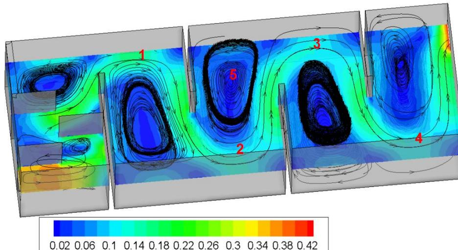
Figure 2: Contour of velocity magnitude [m/s], and some pathlines of water are highlighted. The numbers refer the points, where the water age is determined during the calculation
