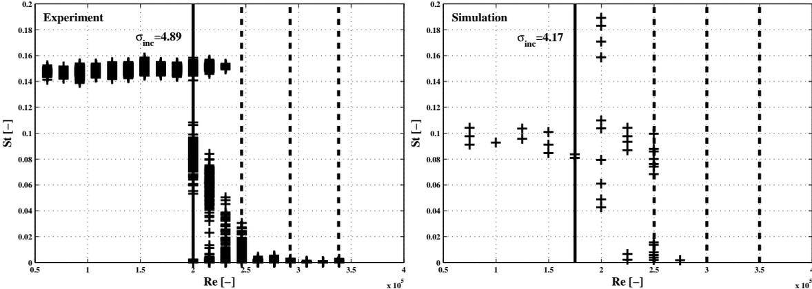
**Figure 2.1:** The comparison of the Reynolds number - Strouhal number relationship of the experiment ( $H = 25$  mm) and the numerical simulation.
