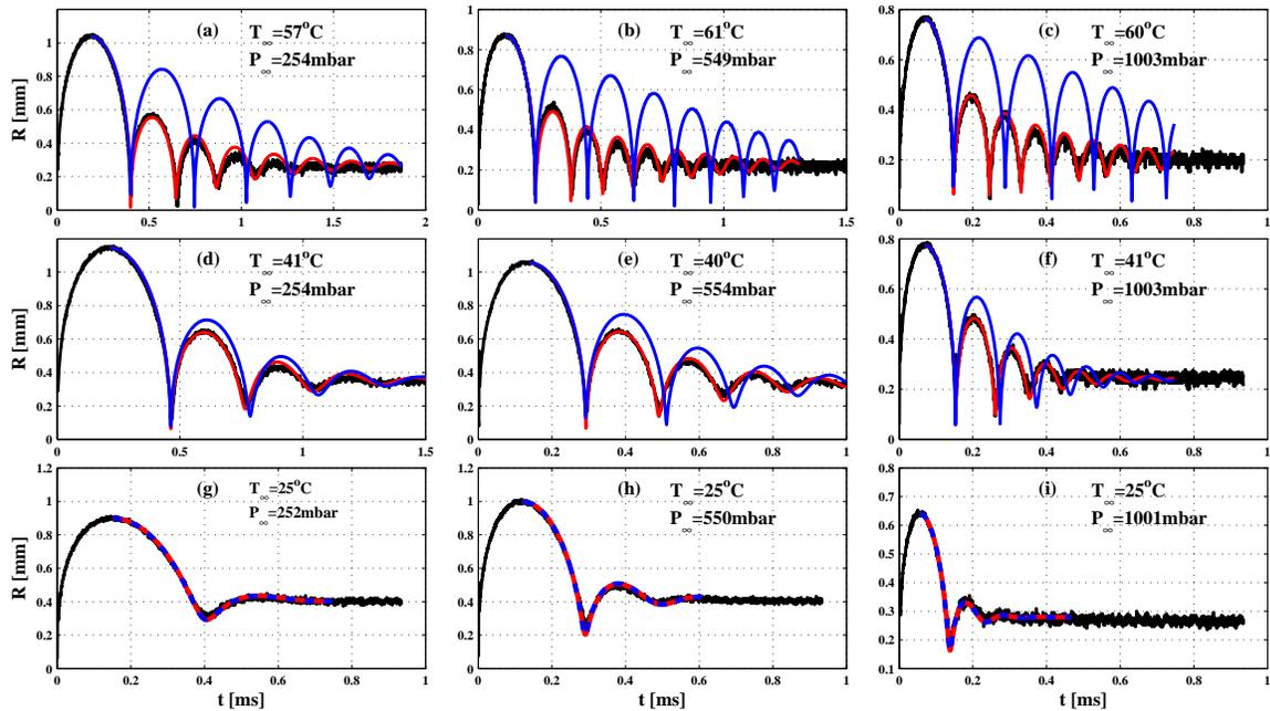
**Figure 1.2:** Comparison of the measurement and the results obtained from the models at different temperature and pressure values. The black, red and blue curves are the results of the measurement, Keller–Miksis and Rayleigh–Plesset equation, respectively. In subfigures (a) to (c) the black and the red lines are nearly congruent.
