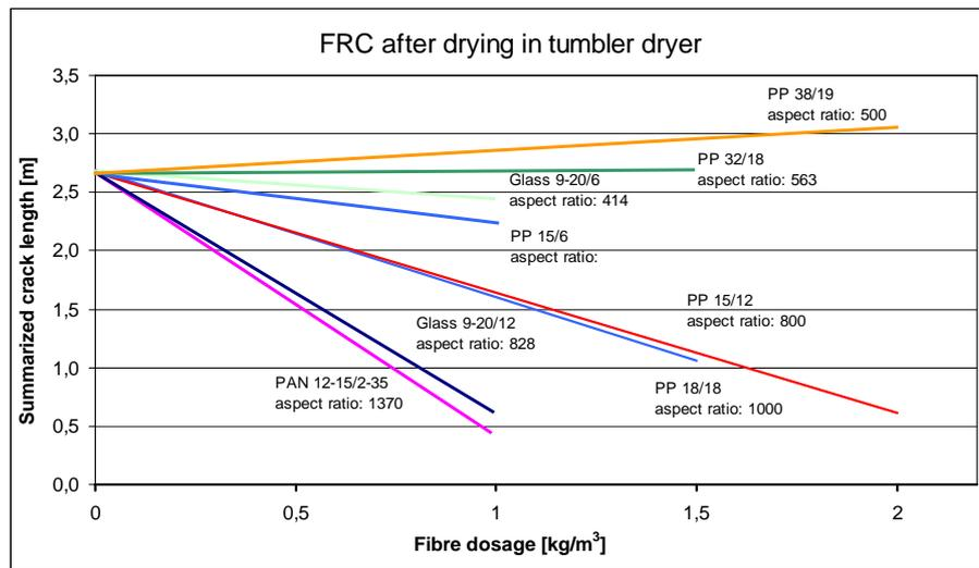
Fig. T6. Relationship between effectiveness of reducing early age shrinkage cracking tendency (average summarized crack lengths of four specimens) of fibres and the fibre aspect ratio
