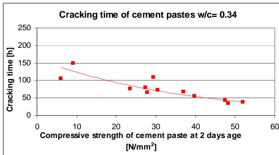
Fig. T8. Relationship between cracking time of the cement paste rings and the compressive strength of the cement paste prisms at the age of 2 days (average of three specimens, w/c = 0.34)
