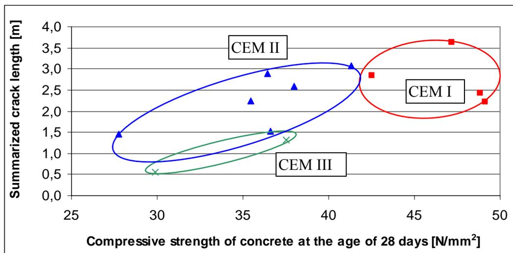
Fig. T19. Relationship between early age shrinkage cracking tendency of concretes (average of four specimens) and the compressive strength of concrete cubes at the age of 28 days (average of three specimens, w/c = 0.61) using different cement types
