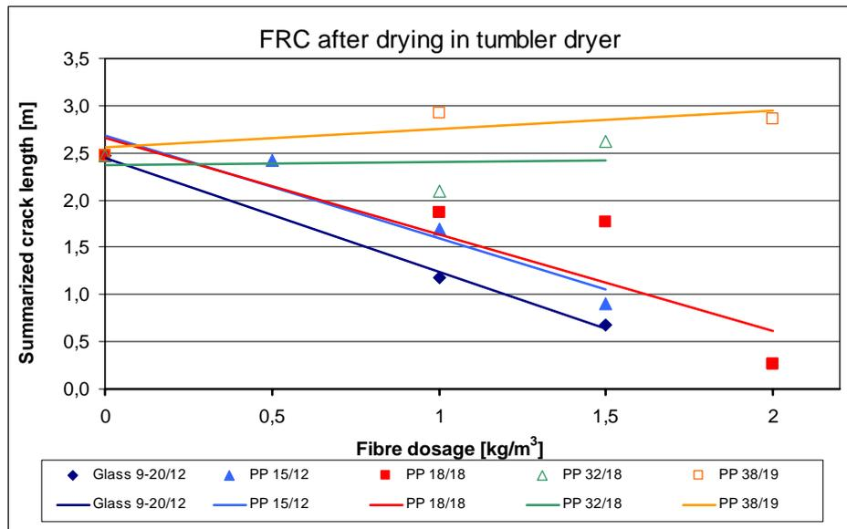
Fig. T3. Relationship between early age shrinkage cracking tendency (average summarized crack lengths of four specimens) of FRC after curing in tumbler drier and the fibre dosage
