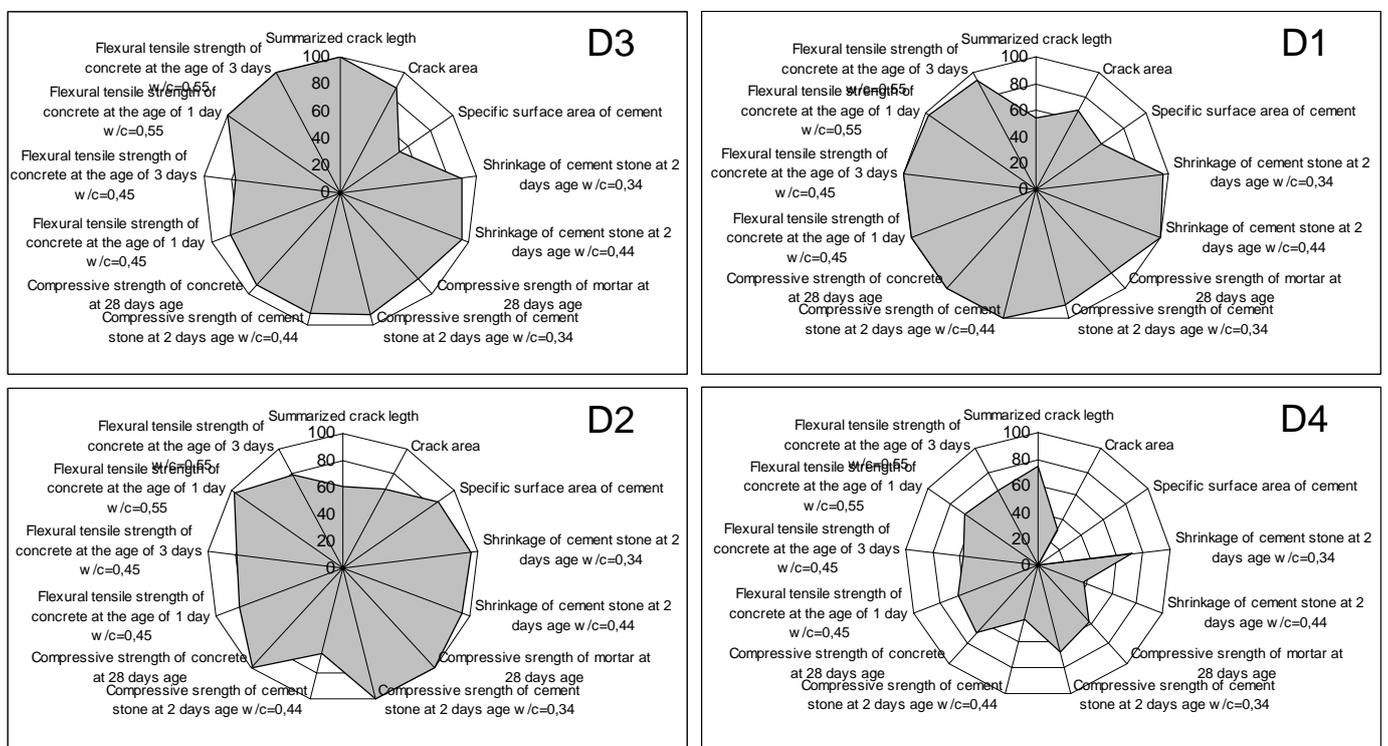
Fig. T12. Relationships between CEM I cement type, and crack length and crack area sorted by the early age shrinkage cracking tendency
