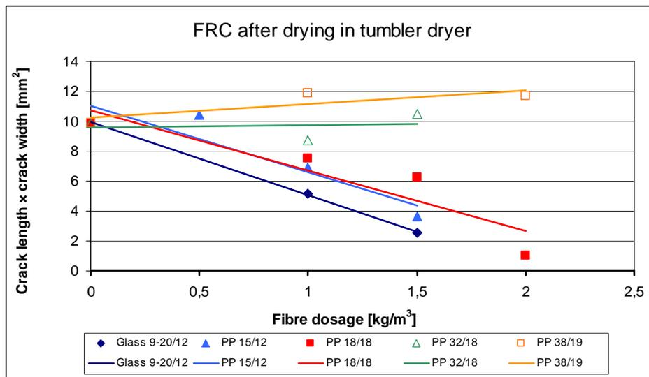
Fig. T4. Relationship between early age shrinkage cracking tendency (summarized crack lengths × crack width, average of four specimens) of FRC after curing in tumbler drier and the fibre dosage
