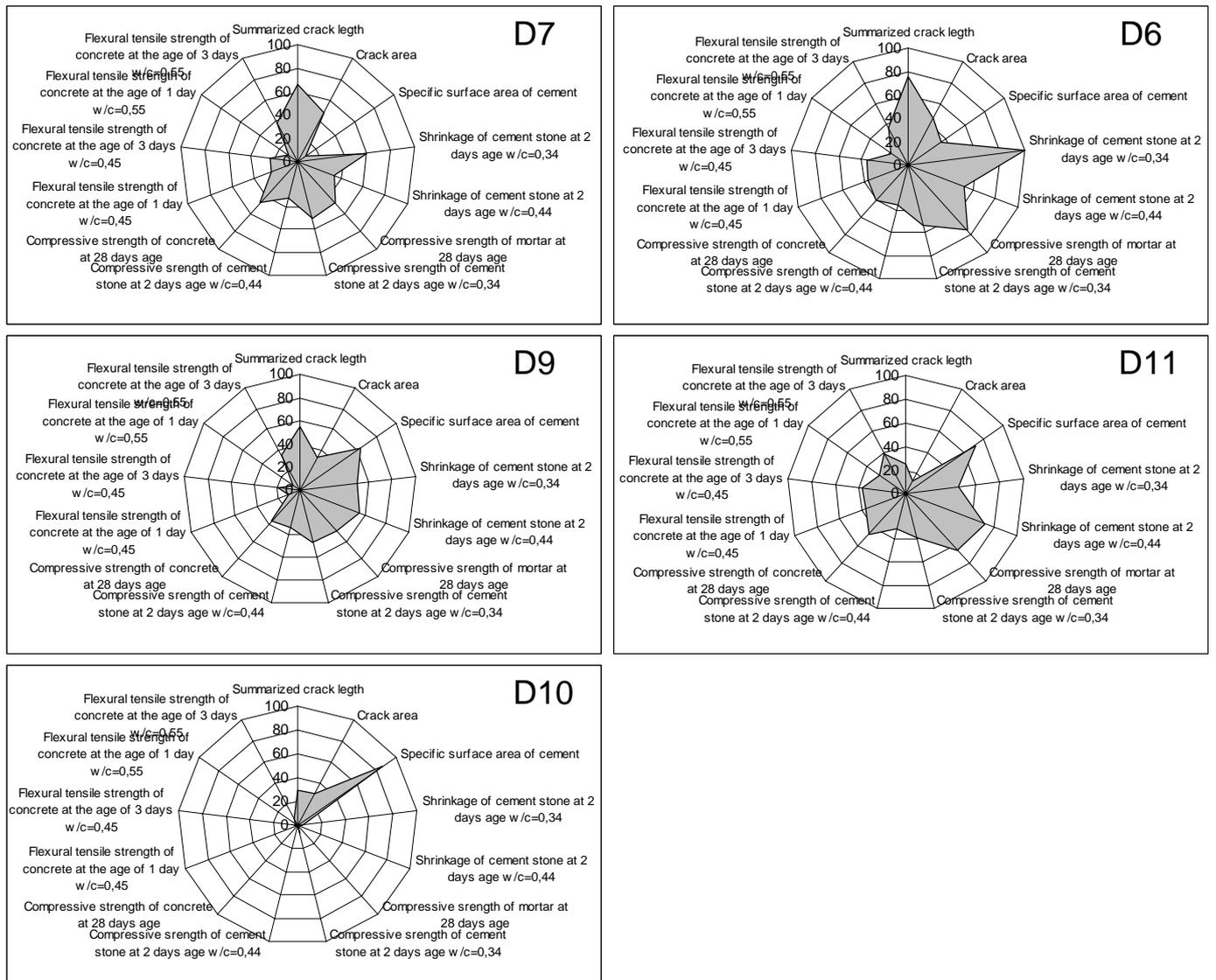
Fig. T13. Relationships between CEM II cement type, and crack length and crack area sorted by the early age shrinkage cracking tendency
