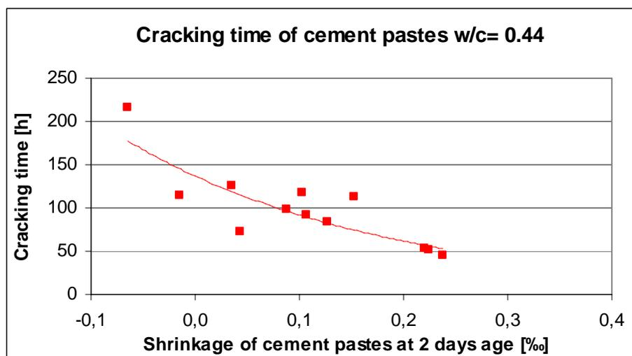
Fig. T11. Relationship between cracking time of the cement paste rings (average of three specimens,  $w/c = 0.44$ ) and the shrinkage of cement paste prisms at the age of 2days (average of three specimens,  $w/c = 0.44$ )
