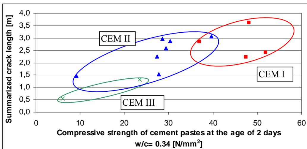
Fig. T16. Relationship between early age shrinkage cracking tendency of concrete rings (average of four specimens) and the compressive strength of the cement paste prisms at the age of 2 days (average of three specimens, w/c = 0.34) using different cement types
