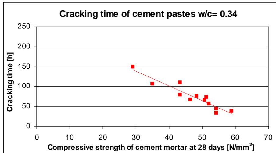
Fig. T9. Relationship between cracking time of the cement paste rings (average of three specimens, w/c = 0.34) and the compressive strength of the cement mortar prisms at the age of 28 days (average of three specimens, w/c = 0.50)
