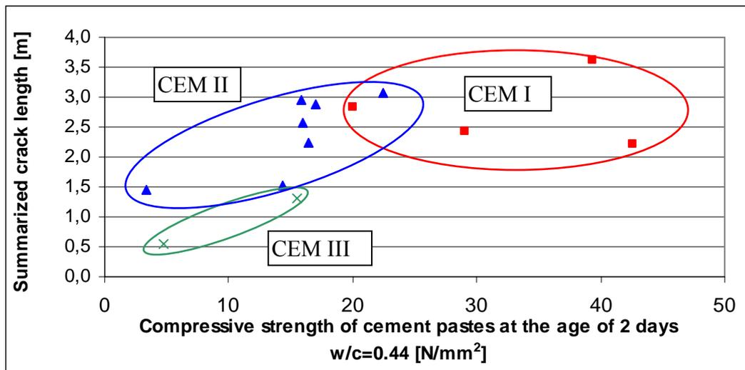
Fig. T17. Relationship between early age shrinkage cracking tendency of concrete rings (average of four specimens) and the compressive strength of the cement paste prisms at the age of 2 days (average of three specimens, w/c = 0.44) using different cement types
