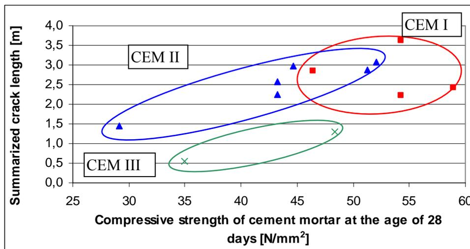
Fig. T18. Relationship between early age shrinkage cracking tendency of concrete rings (average of four specimens) and the compressive strength of the cement mortar prisms at the age of 28 days (average of three specimens, w/c = 0.50) using different cement types
