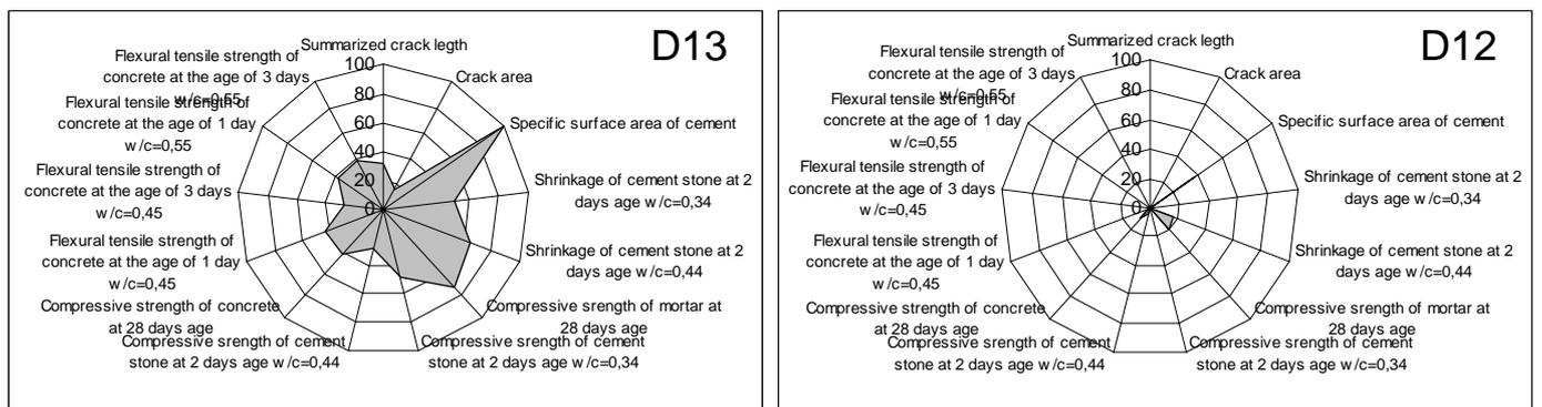
Fig. T14. Relationships between CEM III cement type, and crack length and crack area sorted by the early age shrinkage cracking tendency
