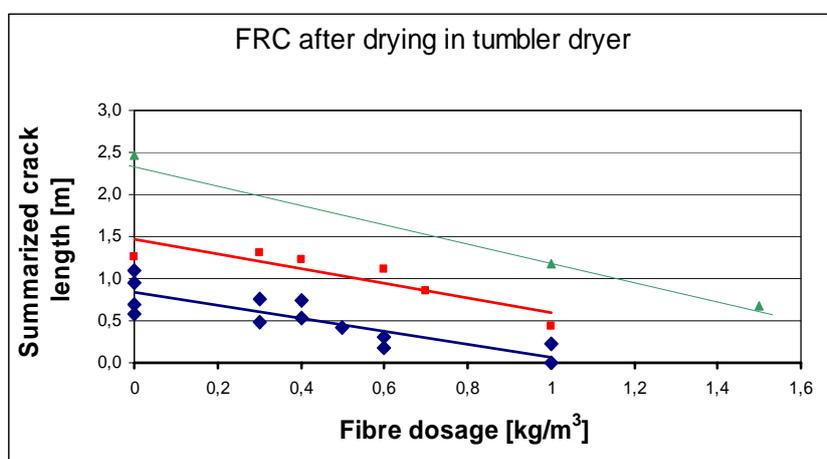
Fig. T7. Relationship between early age shrinkage cracking tendency of glass fibre reinforced concretes (average summarized crack lengths of four specimens) after curing in tumbler drier and the fibre dosage with different cracking tendency of reference mixtures (made without fibres)
