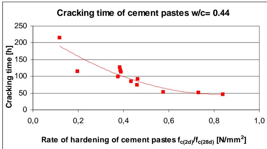
Fig. T10. Relationship between cracking time of the cement paste rings (average of three specimens,  $w/c = 0.44$ ) and the rate of hardening of the cement paste prisms at the age of 2days/28 days (average of three specimens,  $w/c = 0.44$ )
