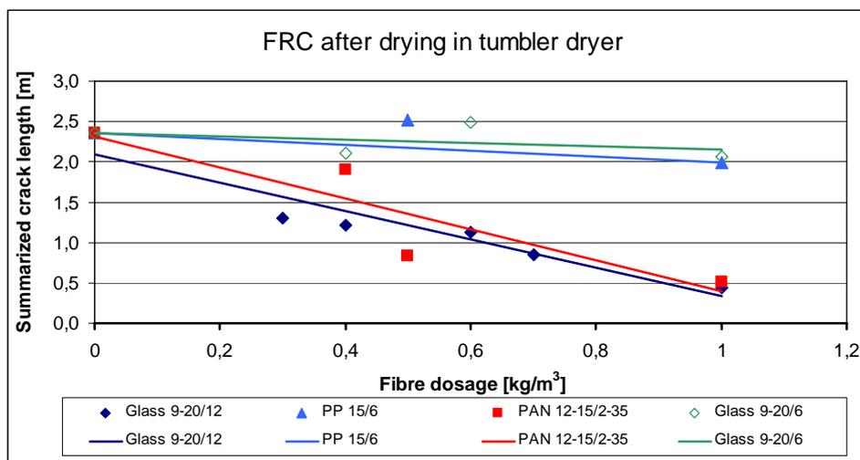
Fig. T5. Relationship between early age shrinkage cracking tendency (average summarized crack lengths of four specimens) of FRC after curing in tumbler drier and the fibre dosage
