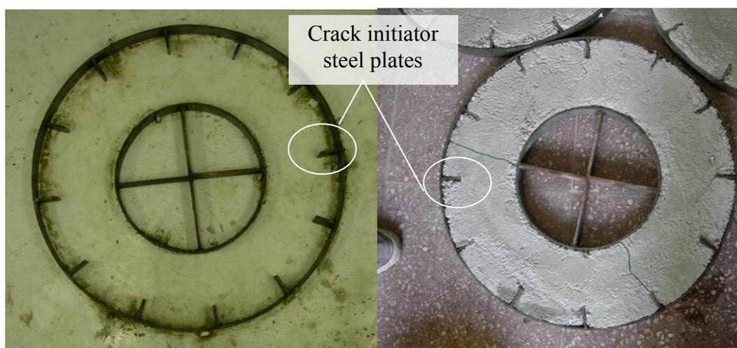
*Fig. 3. Empty (left) and filled (right) formworks for measuring crack tendency*
