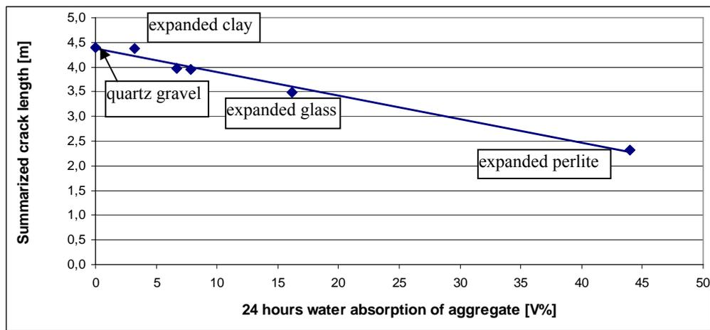
Fig. T1. Relationship between 24 hours water absorption of aggregate and summarized crack length of LWACs after the two (wind tunnel and tumbler dryer) tests (every point indicates the average result of 4 specimens)
