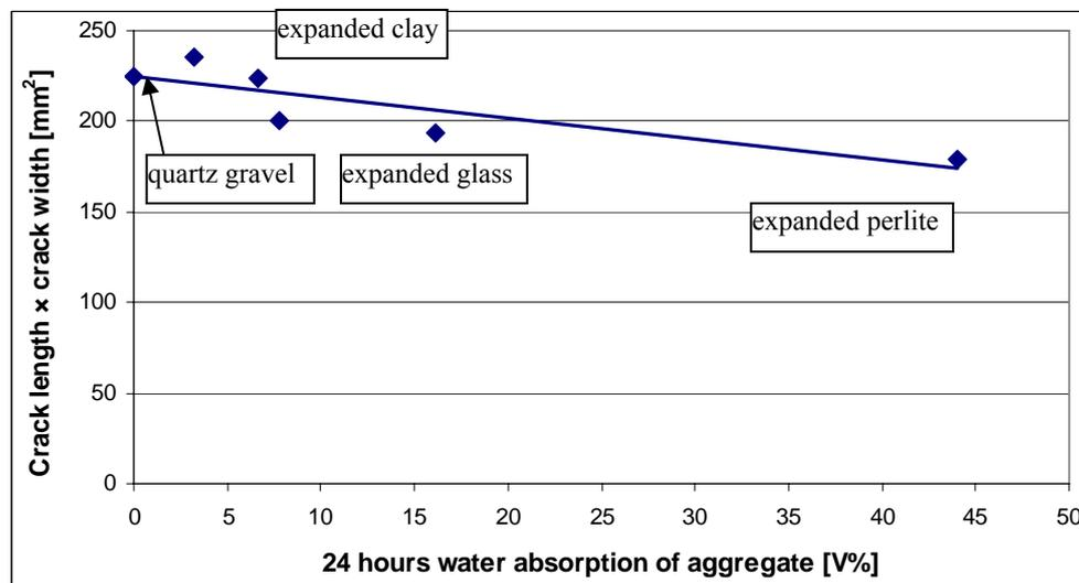
Fig. T2. Relationship between 24 hours water absorption of aggregate and summarized crack length × crack width of LWACs after the two (wind tunnel and tumbler dryer) tests (every point indicates the average result of 4 specimens)
