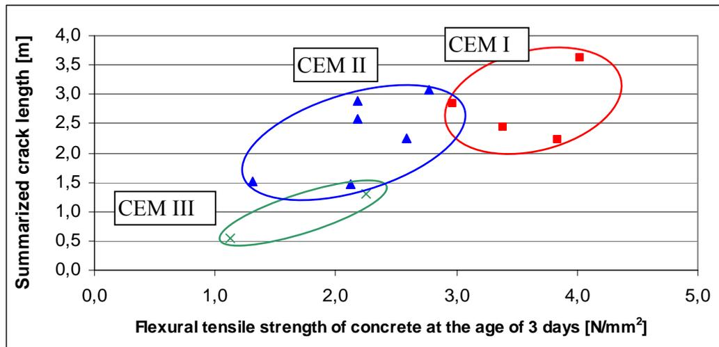
Fig. T15. Relationship between early age shrinkage cracking tendency of concrete rings (average of four specimens) and the flexural tensile strength of concrete prisms at the age of 3 days (average of three specimens, w/c = 0.55) using different cement types
