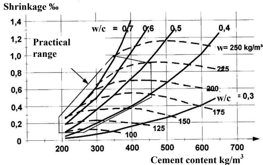
*Fig. 1. Drying shrinkage related to cement content and water-cement ratio [Grube 2003]*
