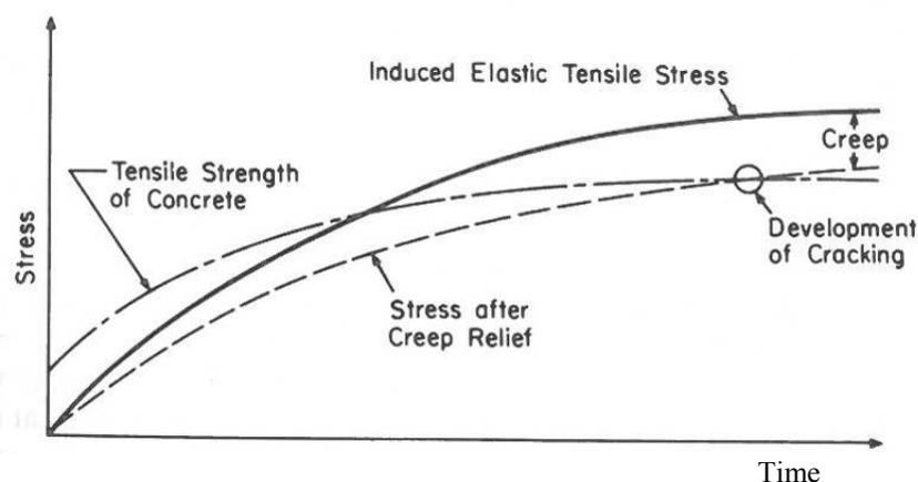
*Fig. 2. Relationship between tensile strength and shrinkage induced tensile stress [Neville 1995]*
