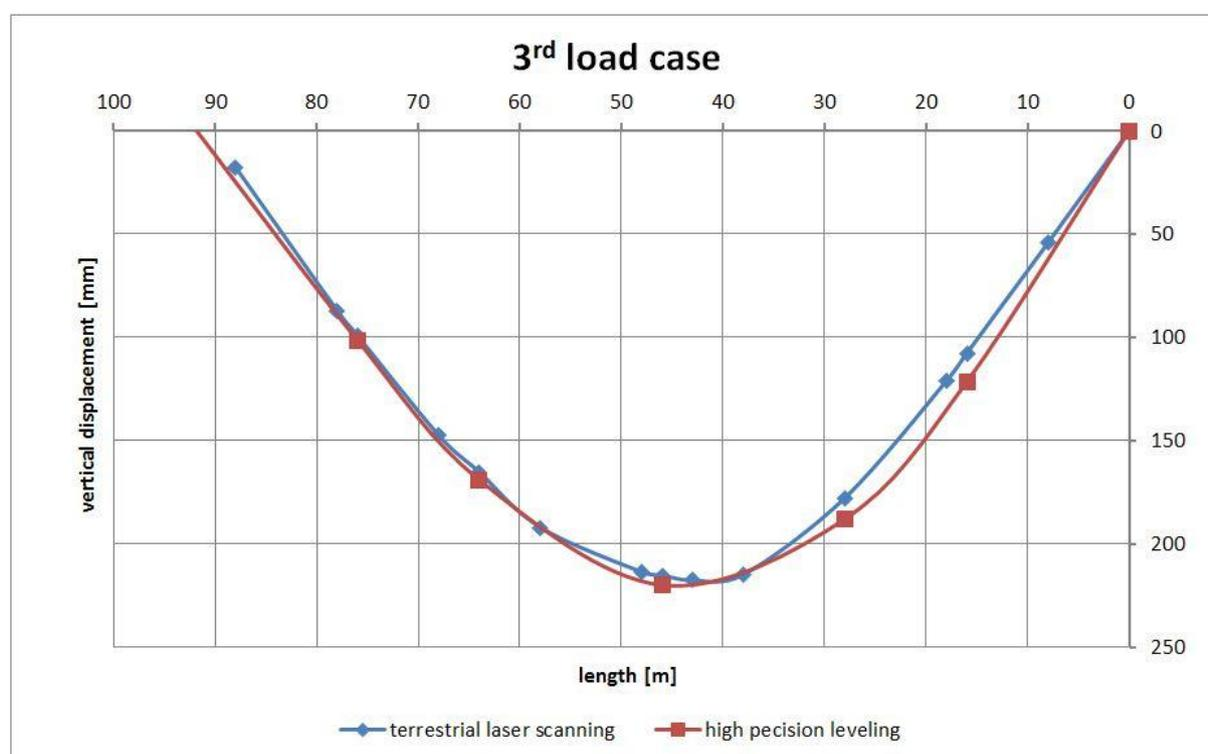
Figure 2: Vertical displacements in the 3<sup>rd</sup> load case of the Szebényi viaduct.
