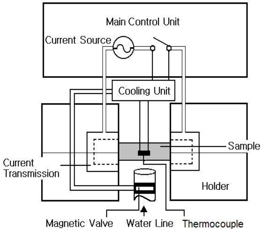
**Figure 3.2. Thermal fatigue device**
