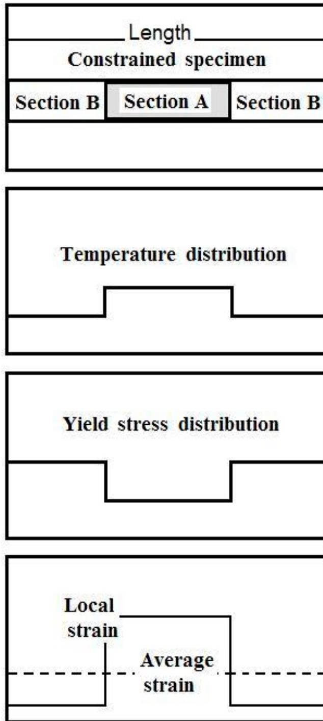
**Figure 2.2. Inducing local strain by yield stress in high temperature region**
