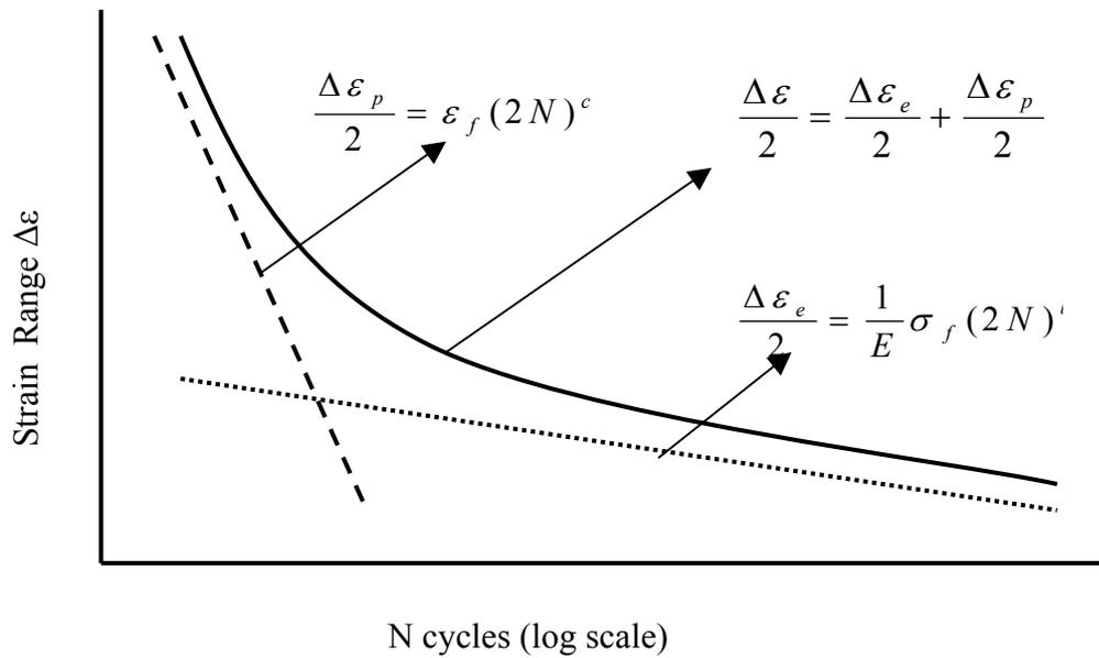
**Figure 2.1. Fatigue strain and life time curve**
