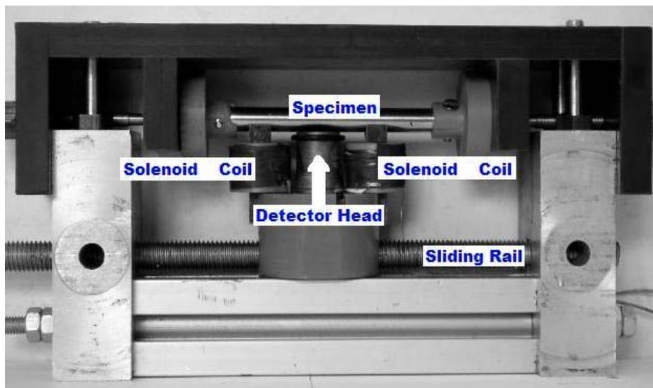
**Figure 3.4. Image of second type BN detect tool**
