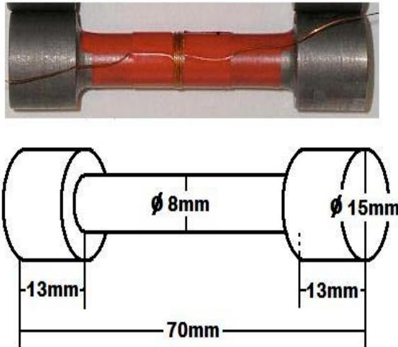
In order to apply repeated thermal fatigue for the system, a special device is used. (See figure 3.2.) This system was designed so that the specimen can be inserted or be picked up with the holder. If the specimen is loaded to the thermal fatigue device (Fig. 3.2.) with the holder, the specimen is fixed by the holder during the thermal fatigue process and thermal strain happens only in the specimen
