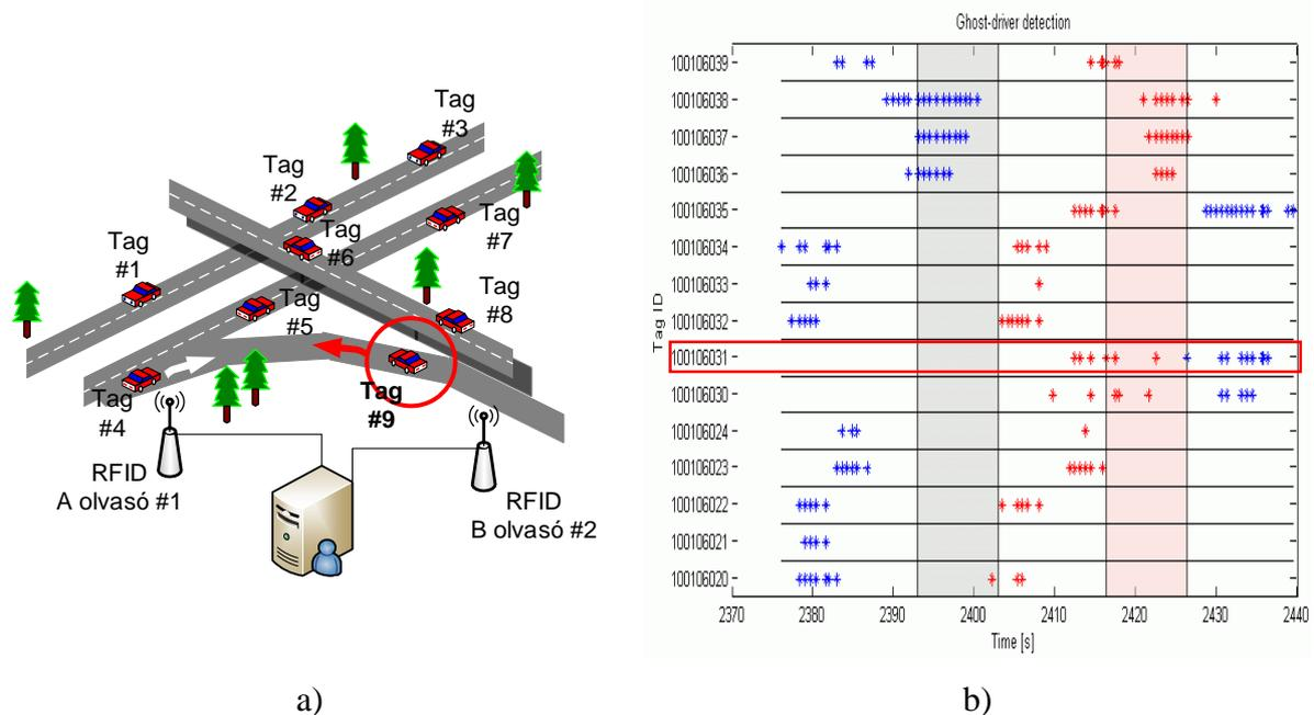
Fig. 3: a) Schematic illustration of detecting wrong way driver
