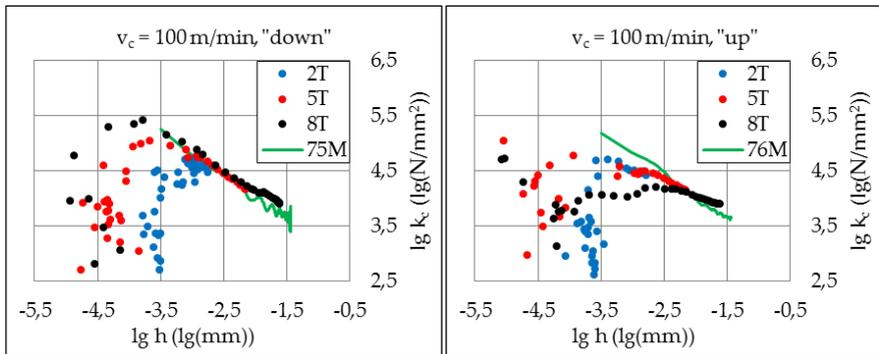
Fig. 5. Comparison of specific cutting forces acquired from milling and turning tests
