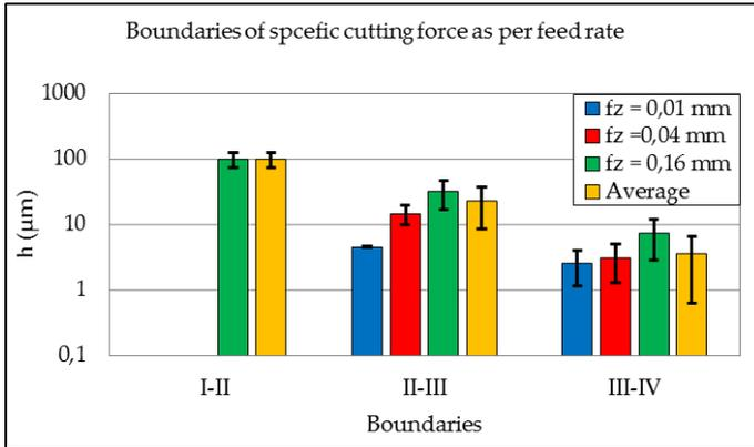
Fig. 3. Section boundaries of cutting force as per feed rate
