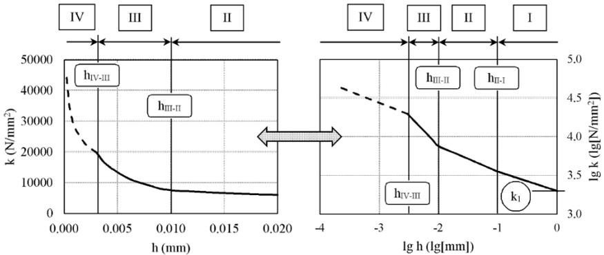
Fig. 1.: Multi-partitioned model of specific cutting force [B1, pp. 2737]
