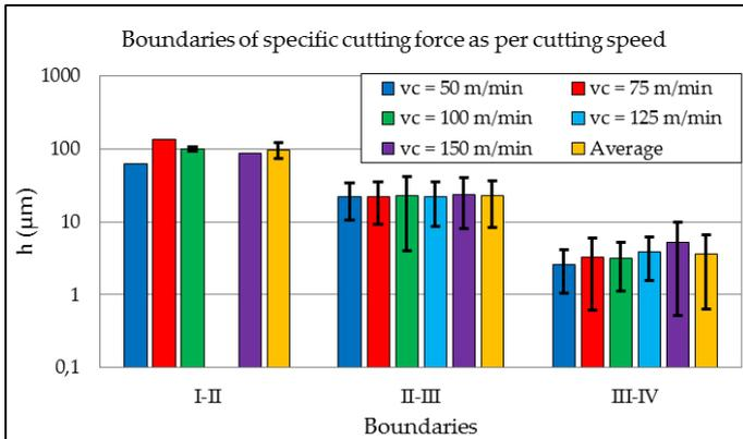
Fig. 4. Section boundaries of cutting force as per cutting speed
