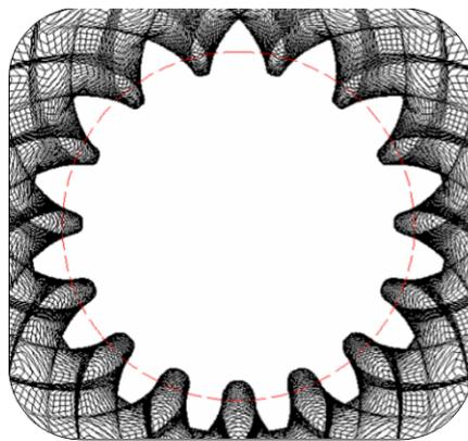
4. **Thesis:** The numerically generated gear geometry consists of numerous line segments. After importing these into 3D CAD systems the work may be cumbersome. Spline curves can only be laid on continuous line segments. I created an algorithm that can automatically detect and separate each curve segment of the teeth such as flank curves, undercut curves top land and bottom land curves. For this purpose the numerically determined curvature functions were used.
