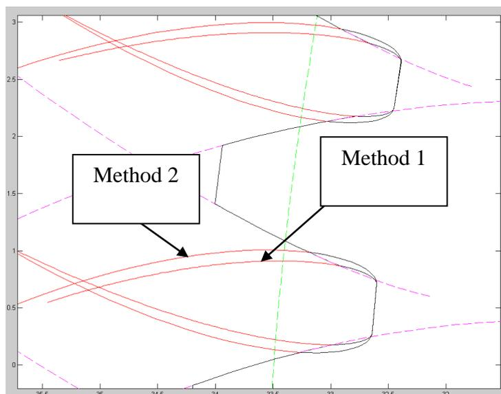
Figure 9. The resulting undercut curves
