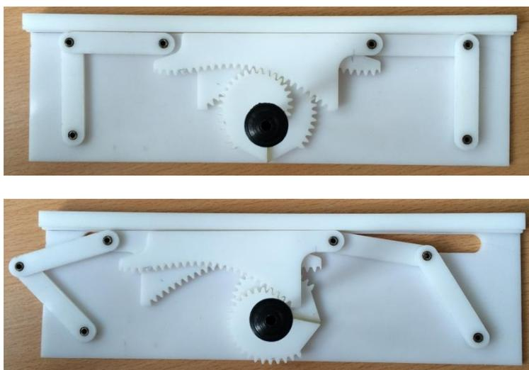
Figure 6. The 2D mockup in initial and deflected position.
