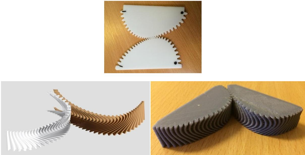
*Figure 10. The generated and manufactured gears*
