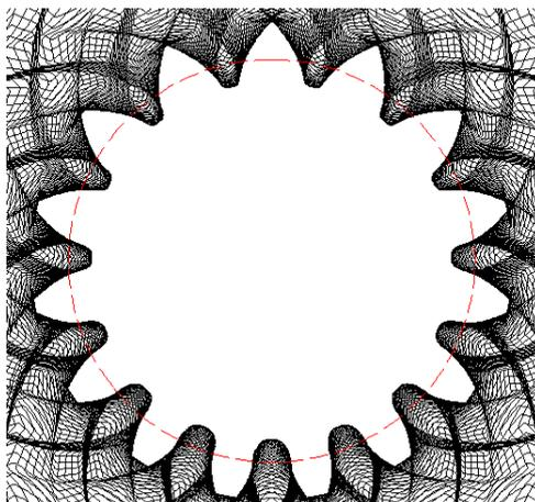
Figure 8. A cylindrical gear with changing profile shift
