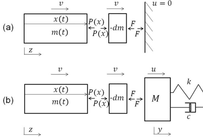
Fig. 2: (a) Original and (b) elastic Riera model
