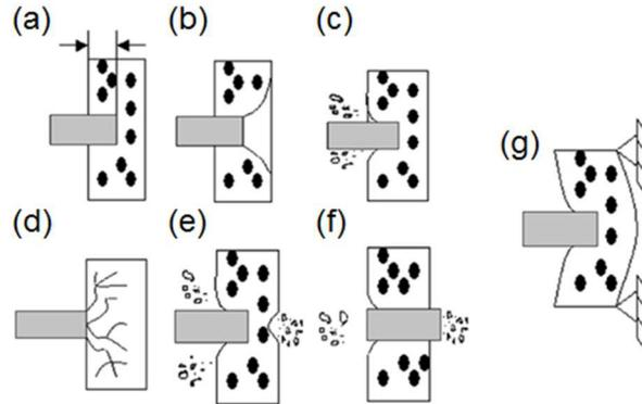
Fig. 1: Local effects: (a) penetration, (b) cone cracking, (c) spalling, (d) cracks, (e) scabbing, (f) perforation and global effect (g) of missile impact (Li et al., 2005)
