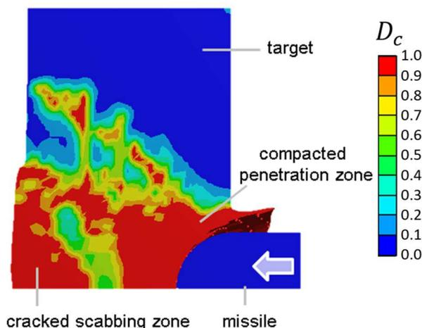
Fig. 6: Damage of concrete target in the FE model. Red colour represents the totally damaged elements (level of damage,  $D_c=1$ ), blue colour shows the intact parts ( $D_c=0$ ).
