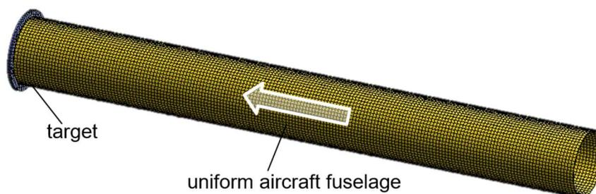
Fig. 3: FE model of uniform aircraft fuselage and rigid target plate
