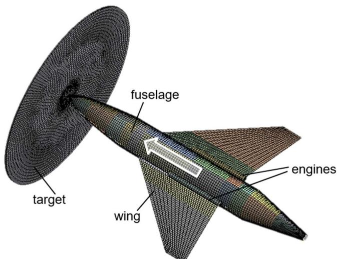
Fig. 5: FE model of aircraft
