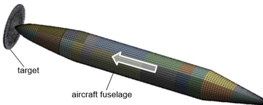
Fig. 4: FE model of aircraft fuselage with nose and tail
